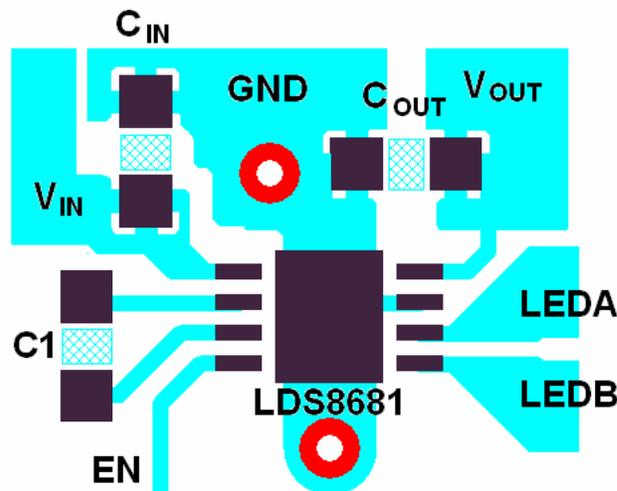
ground plane on the bottom layer through two vias to improve power dissipation.
