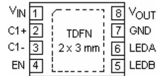
Top view: TDFN 8-lead 2 X 3 mm
