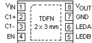
LEDs at 400 mA each simultaneously or one LED at 800 mA. Low dropout PowerLite™ Current Regulator (PCR) increases device's efficiency up to 90%.
