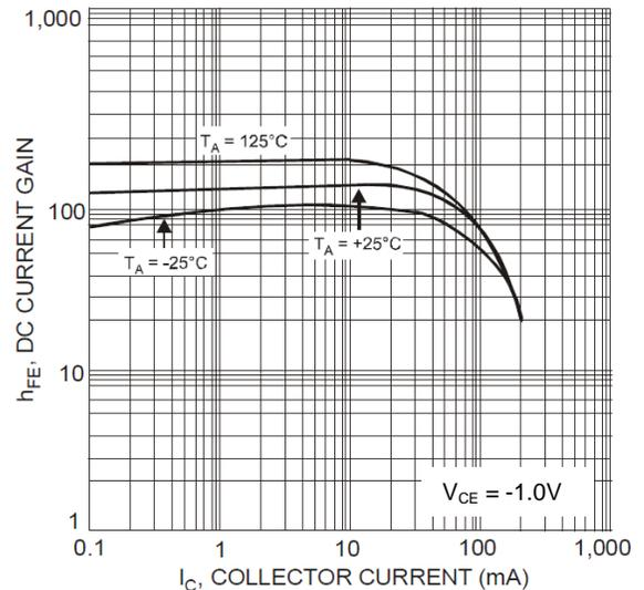
Fig. 3, Typical DC Current Gain vs. Collector Current
