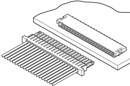
This is an ultra-thin 1.0 mm pitch wire-to-board connector for thinner and smaller devices, with a mounting height of 1.8 mm for the normal type and 1.4 mm for the offset type.
