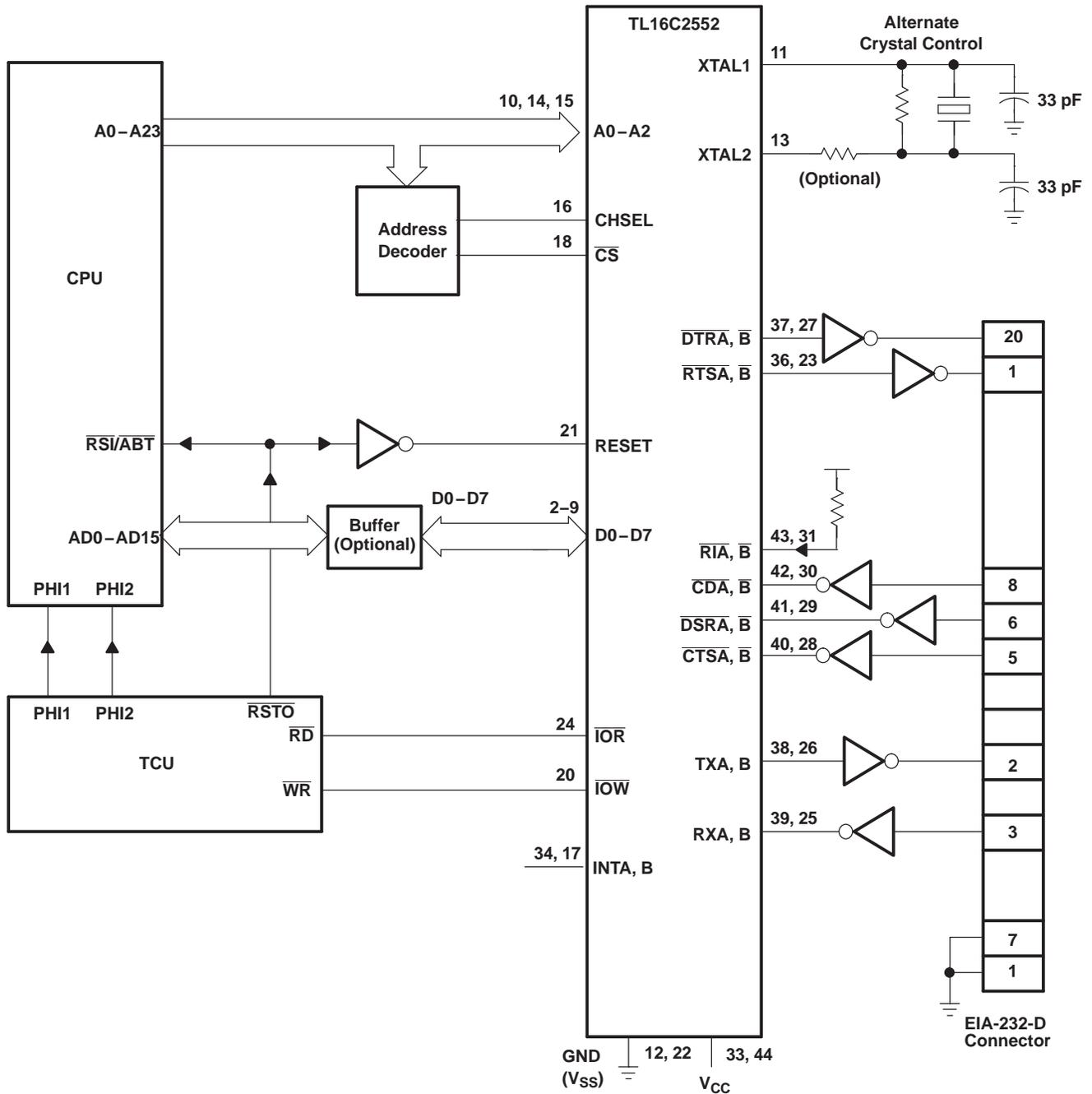
A. Pin numbers shown are for 44-pin PLCC FN package.
