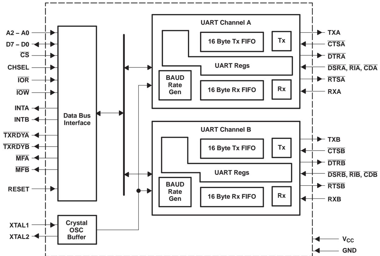
A.  $\overline{MF}$  output allows selection of  $\overline{OP}$ ,  $\overline{BAUDOUT}$ , or  $\overline{RXRDY}$  per channel.
