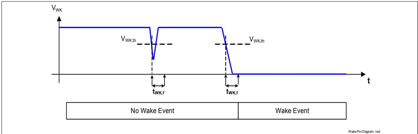
Figure 17 Wake-up Timing
