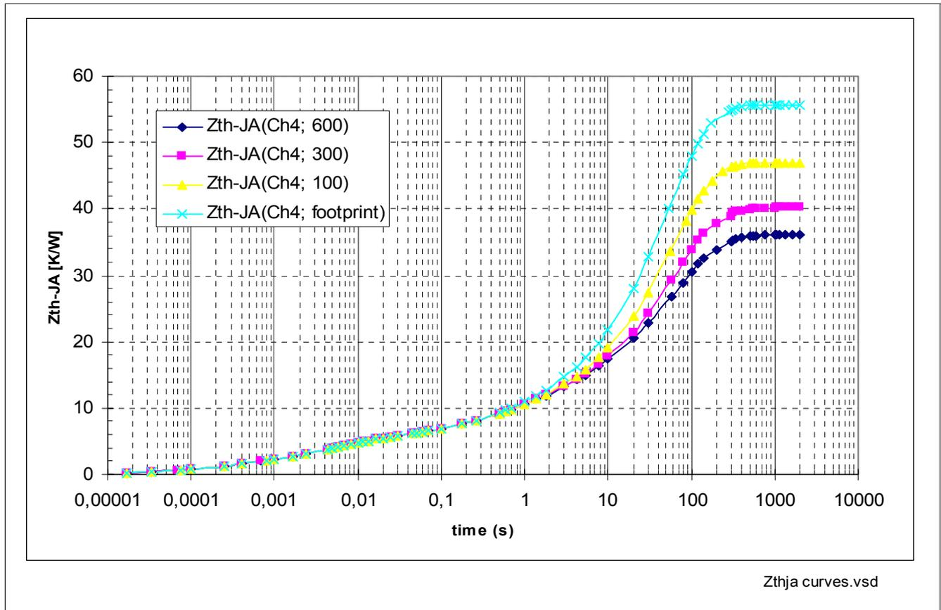
Figure 41 ZthJA Curve, Function of Cooling Area
