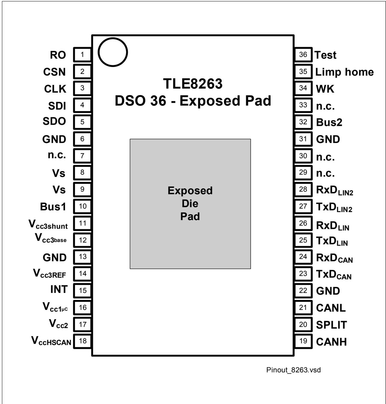
Figure 2 Pin Configuration
