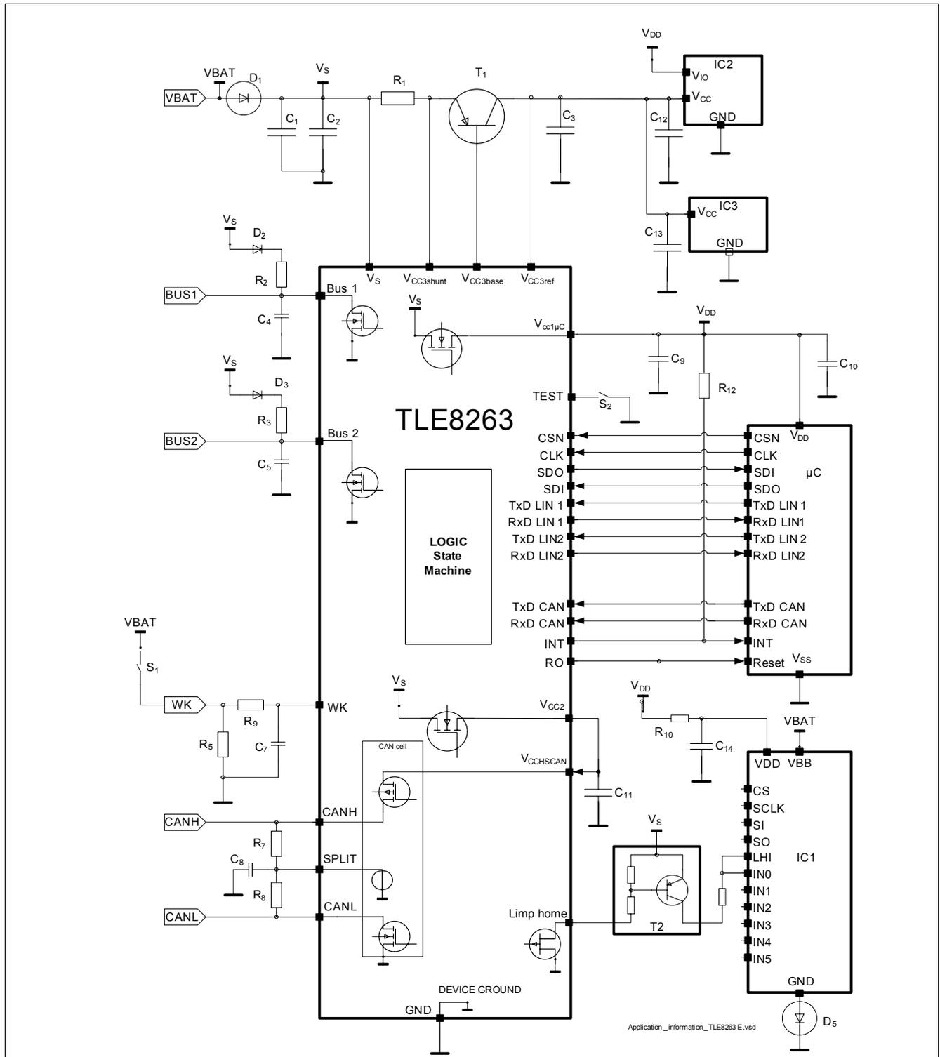
Figure 40 Application Example for a Body Controller Module
