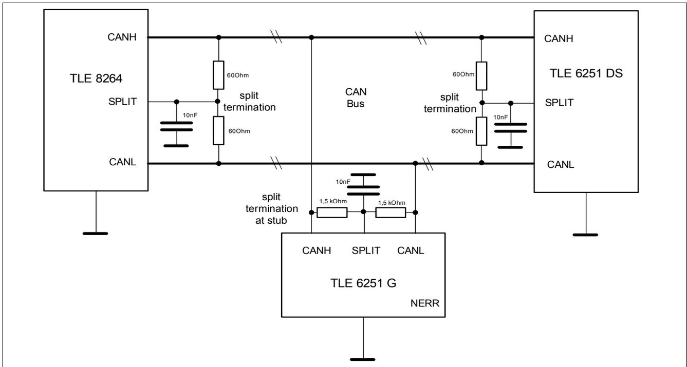
Figure 14 Application example for the SPLIT Pin
