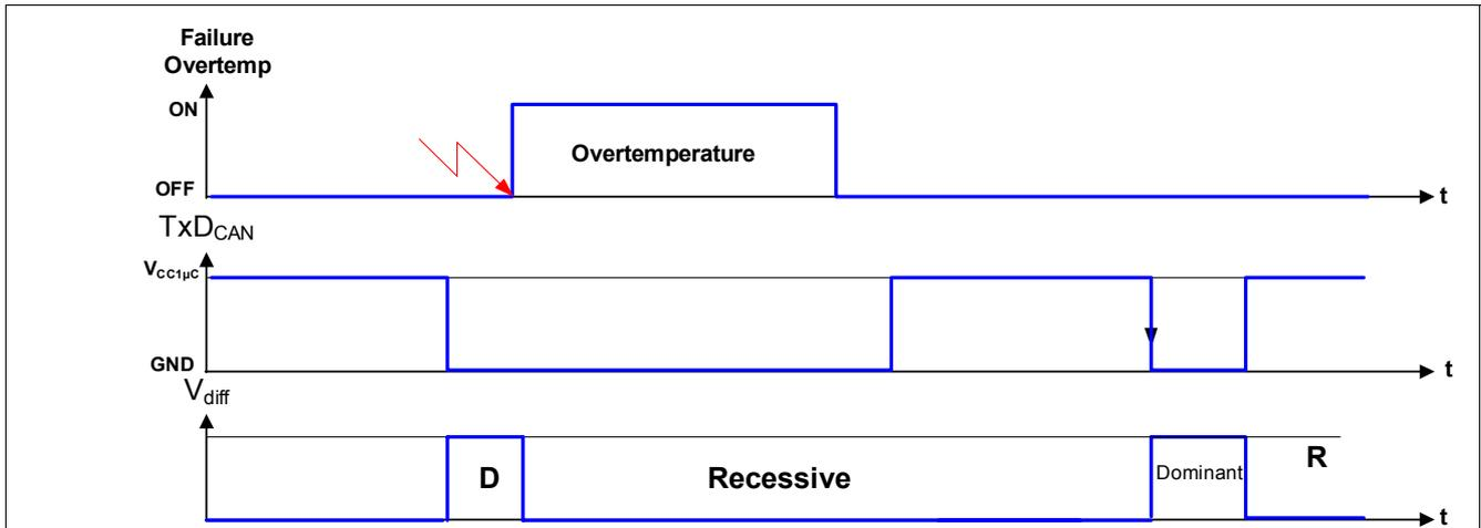
**Figure 13 Release of the Transmission after Overtemperature**
