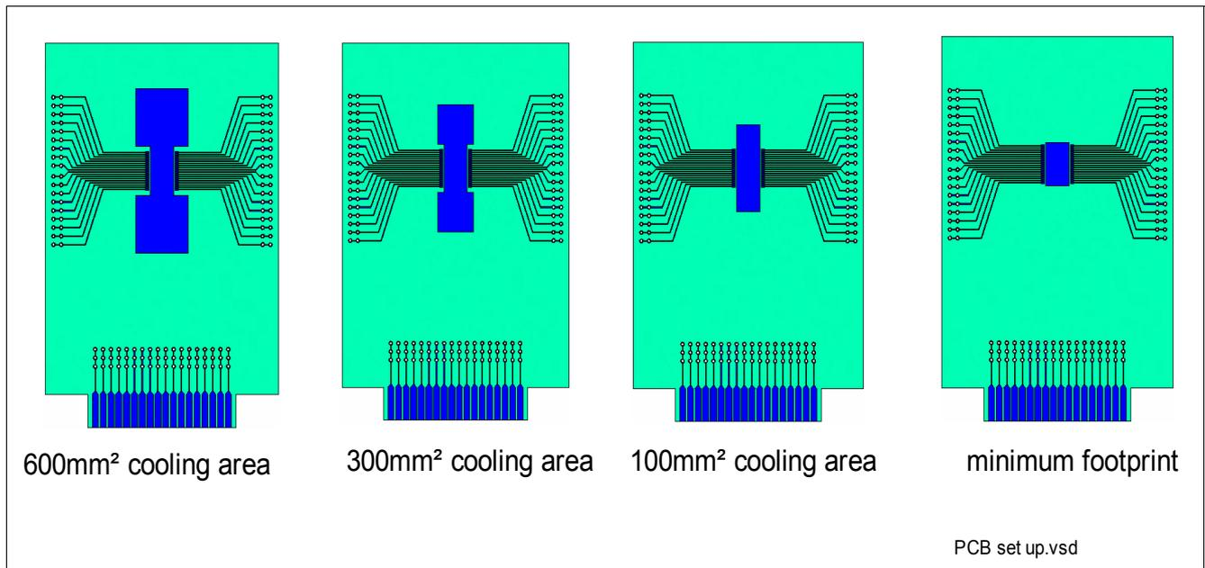
Figure 42 Board Set-up
