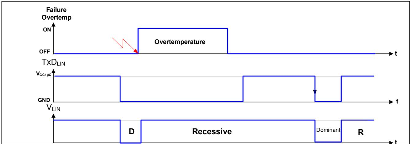
Figure 21 Release of the Transmission after Overtemperature
