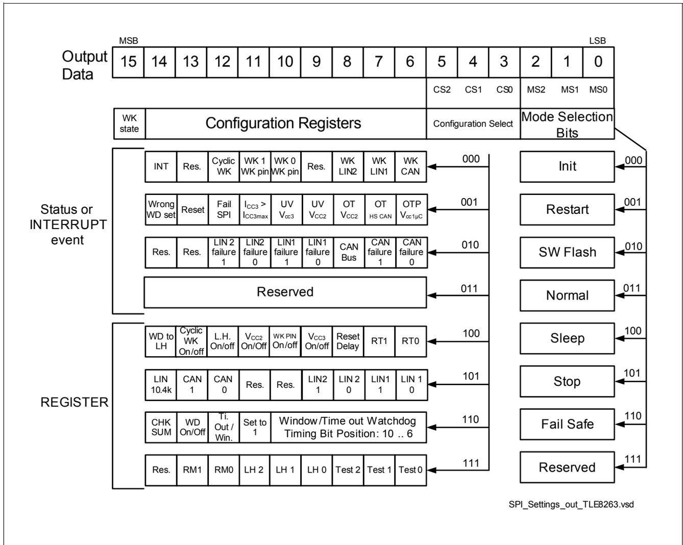
Figure 36 16-bit SPI Output Data / Control Word
