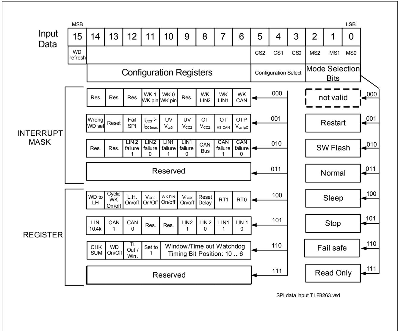
Figure 35 16-Bit SPI Input Data / Control Word
