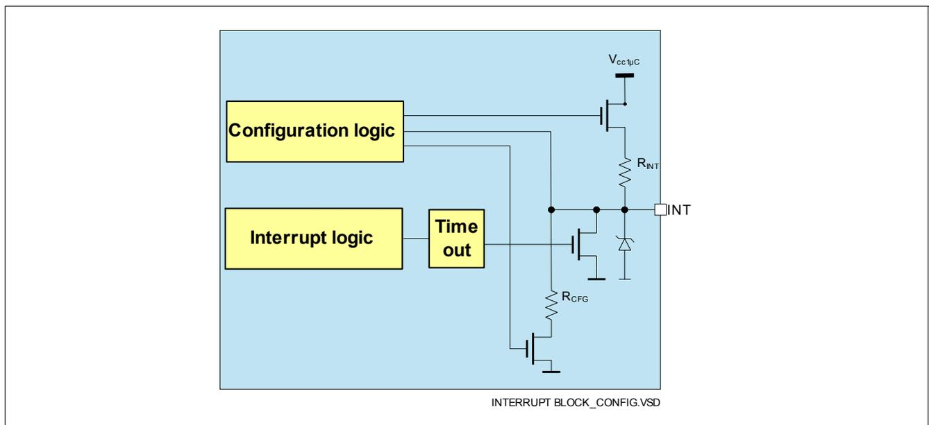
**Figure 33** Config Logic Diagram
