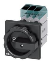
Load disconnector 3LD3, lu 40 A Main switch 3-pole Rated operating capacity at AC-23 A at 400 V 18.5 kW Front plate mounting Basic switch with Central hole mounting 22.5mm Toggle drive black 66x66 mm
