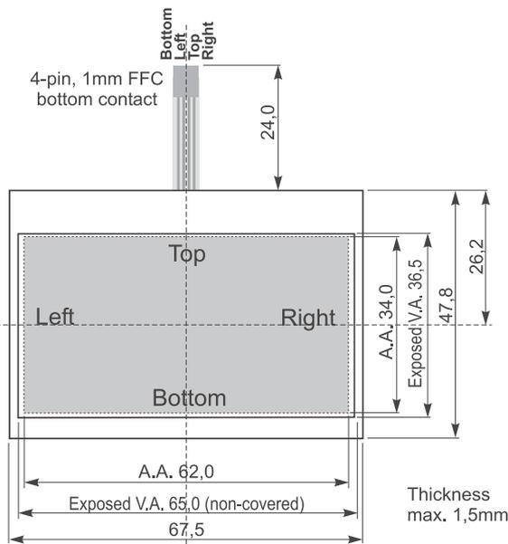
Interfacing to a processor can be either done by an external touch panel controller or with a controller that is featured with analogue input. The touch panel is similar to a potentiometer: connecting a voltage of e.g. 3.3V to the pins *Top-Bottom* makes it possible to read out a voltage on pin *Left* or *Right* which is linear to the Y-coordinate of the pressed point. The X-coordinate will result when the voltage will be supplied to
