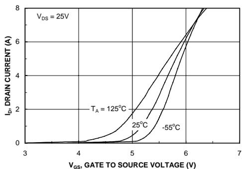
Figure 5. Transfer Characteristics.
