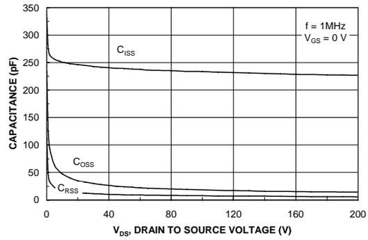
Figure 8. Capacitance Characteristics.
