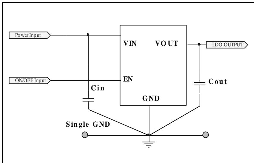
Note:  $C_{in}=C_{out}=1\ \mu F$
