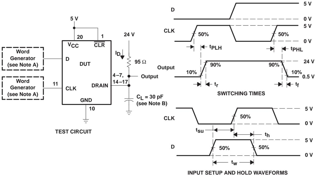
Figure 2. Test Circuit, Switching Times, and Voltage Waveforms
