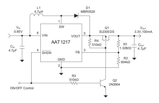
Figure 1: AAT1217 High Efficiency Load Disconnect Application Circuit.
