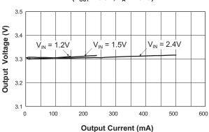
Output Voltage vs. Output Current (V<sub>OUT</sub> = 5V; T<sub>A</sub> = 25°C)
