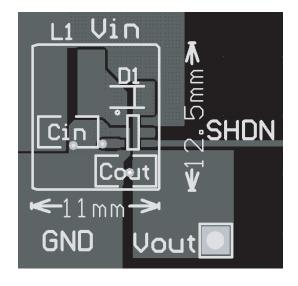
Figure 2: AAT1217 Evaluation Board Layout Example Top Layer.
