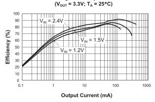
Efficiency vs. Output Current
