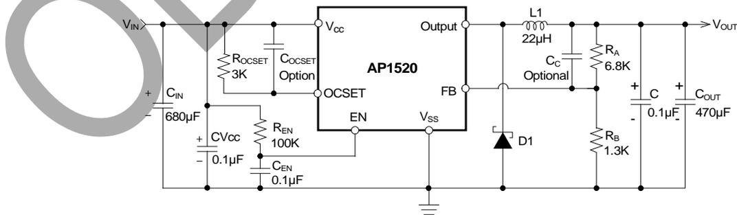
Note:  $V_{OUT} = V_{FB} \times (1 + R_A/R_B)$
