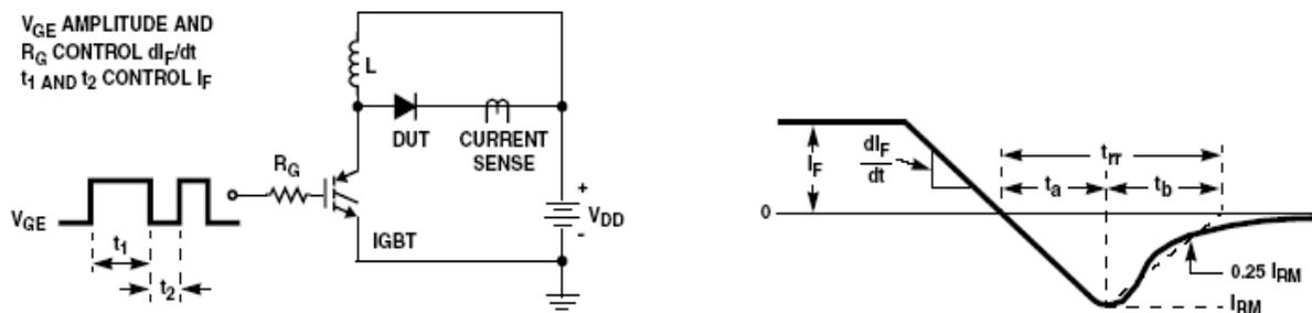
Figure 1. Diode Reverse Recovery Test Circuit & Waveform
