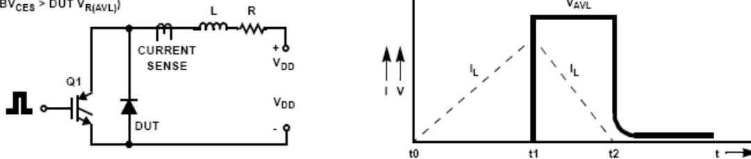
Figure 2. Unclamped Inductive Switching Test Circuit & Waveform
