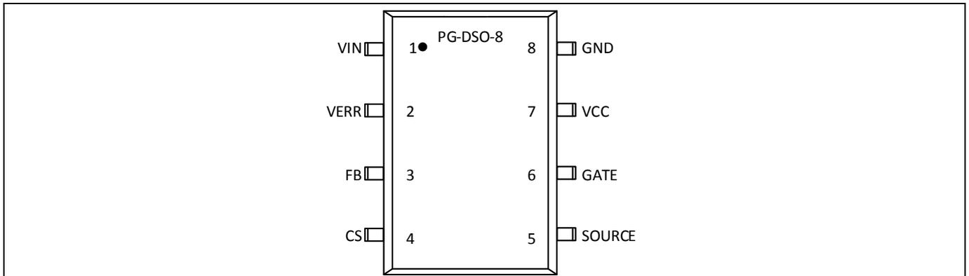
Figure 3 Pin configuration
