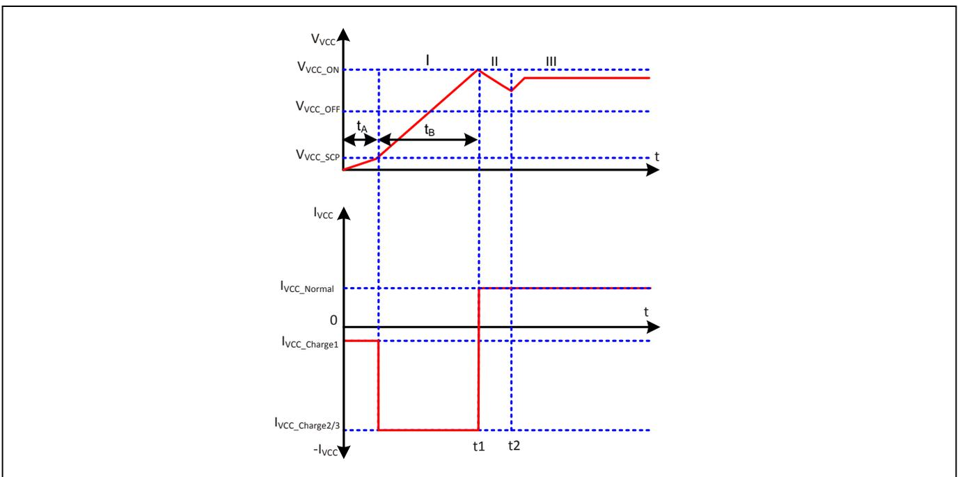
Figure 5 V<sub>CC</sub> voltage and current at startup
