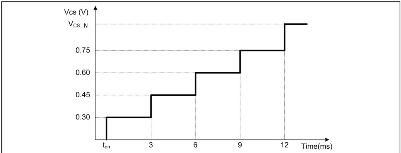
Figure 6 Maximum current sense voltage during soft start
