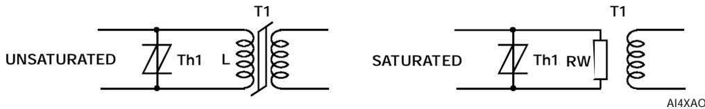
Figure 9. Transformer Saturation
