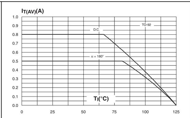
**Figure 3. Average and D.C. on-state current versus ambient temperature (epoxy printed circuit board FR4, copper thickness = 35 μm, S<sub>CU</sub> = 0.5 cm<sup>2</sup>) (TO-92)**
