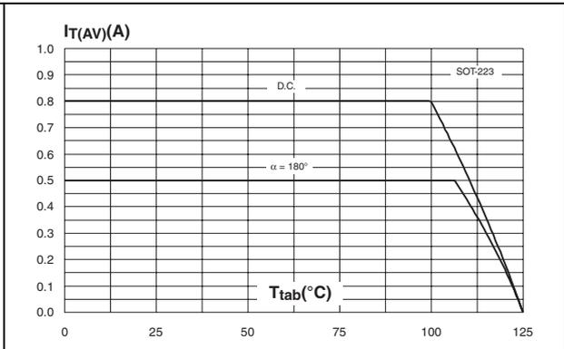
**Figure 5. Average and DC on-state current versus ambient temperature (epoxy PCB FR4, copper thickness = 35 μm, S<sub>CU</sub> = 5 cm<sup>2</sup>) (SOT-223)**
