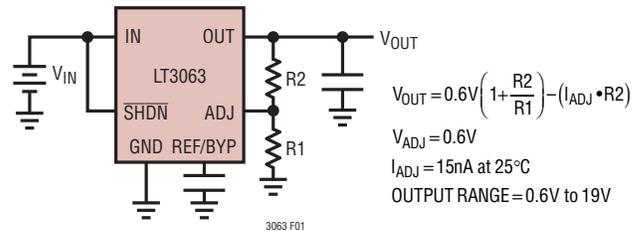
Figure 1. Adjustable Operation
