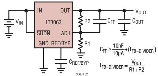
Figure 2. Feedforward Capacitor for Fast Transient Response
