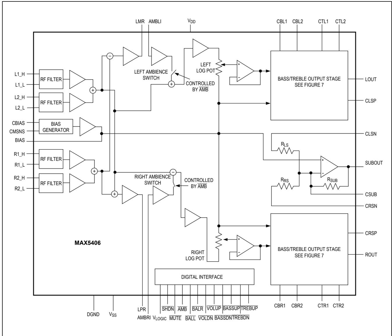
Figure 1. Block Diagram
