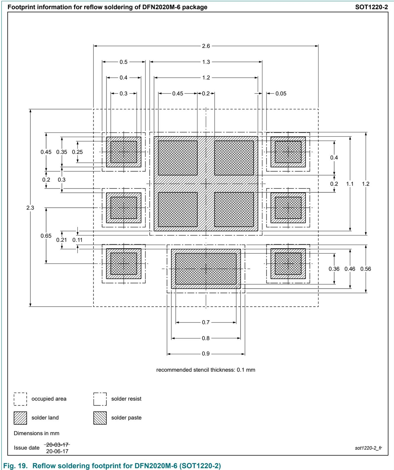
**Fig. 19. Reflow soldering footprint for DFN2020M-6 (SOT1220-2)**
