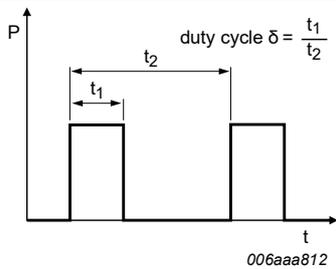
Fig. 17. Duty cycle definition
