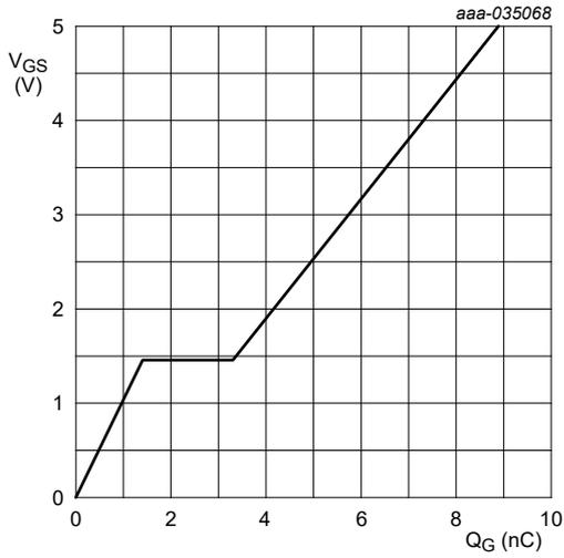
$I_D = 9.3 \text{ A}; V_{DS} = 15 \text{ V}; T_{amb} = 25 \text{ }^\circ\text{C}$
