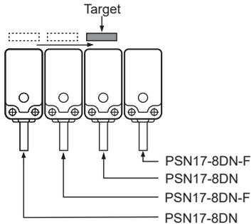
When installing several proximity sensor closely, it may cause malfunction due to mutual interference. Therefore, please use differential frequency for the application
