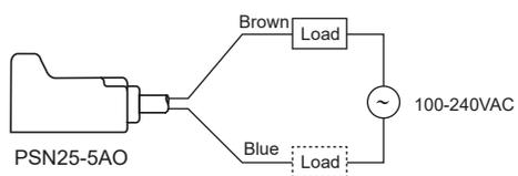
※The load can be connected to either wire.
