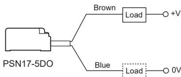
※The load can be connected to either wire.
