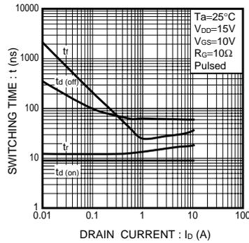
Fig.2 Switching Characteristics
