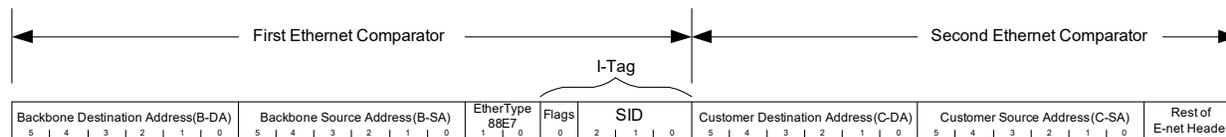
**Figure 43 • PBB Ethernet Frame Format (1 B-Tag)**
