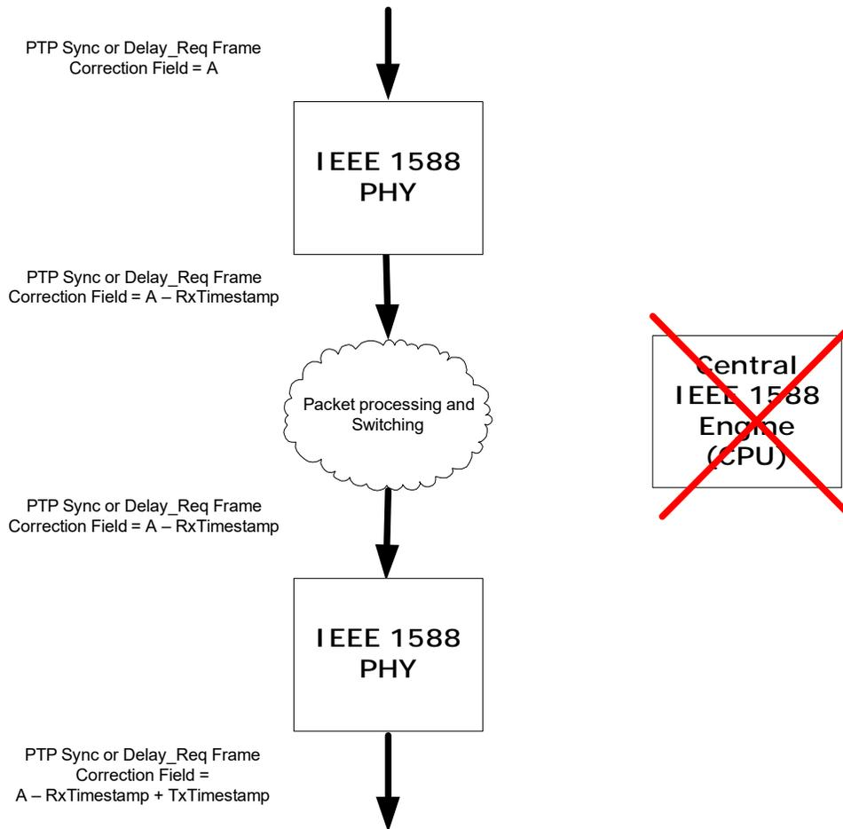
When the system works in one-step E2E TC mode Sync and Delay\_req frames must be forwarded through the system and the residence time = (Egress time stamp – Ingress time stamp) must be added to the correction field in the frame before it leaves the system.
