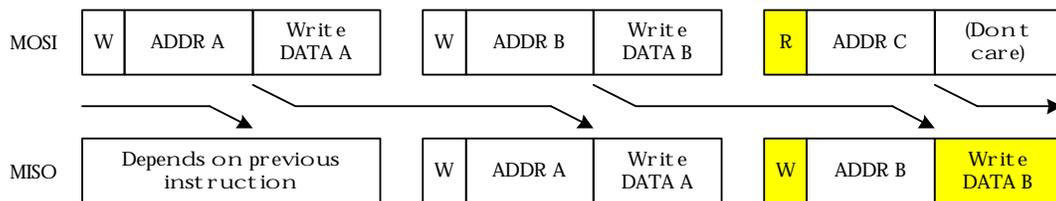
The following illustration shows that when a write instruction follows a read instruction, the MISO data during the write instruction is not pipelined read data. MISO contains all 0's in the data field.
