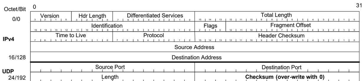
Per flow validation is performed on the Source or Destination Address in the IPv4 header. The comparator can be configured to indicate a match in the flow if the source, destination, or either the source or destination fields match.
