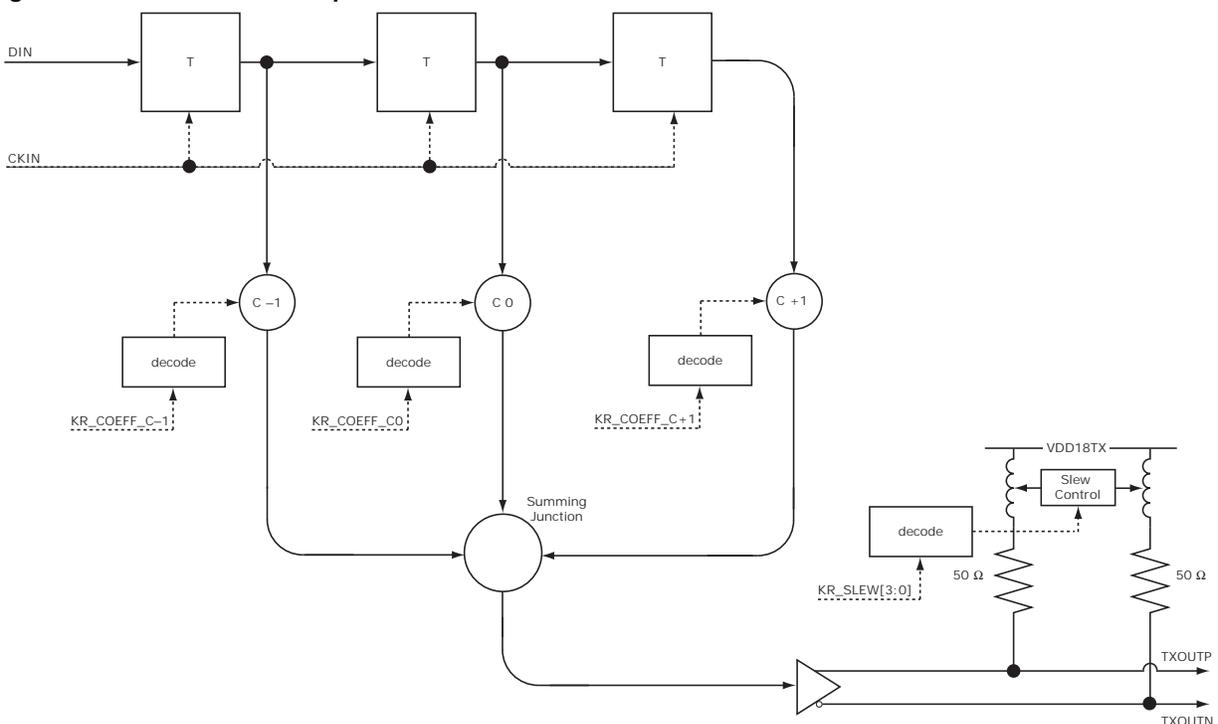
The final output stage has 50  $\Omega$  back-termination with inductor peaking. The output slew rate is controlled by adjusting the effectiveness of the inductors.
