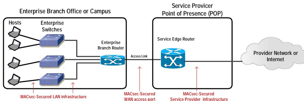
Each host has a dedicated physical link to an Enterprise Ethernet switch, and the switches are connected to an enterprise branch router that also provides WAN access. In smaller configurations, hosts can also connect directly to the branch router. All internal branch office Ethernet ports are secured using MACsec.
