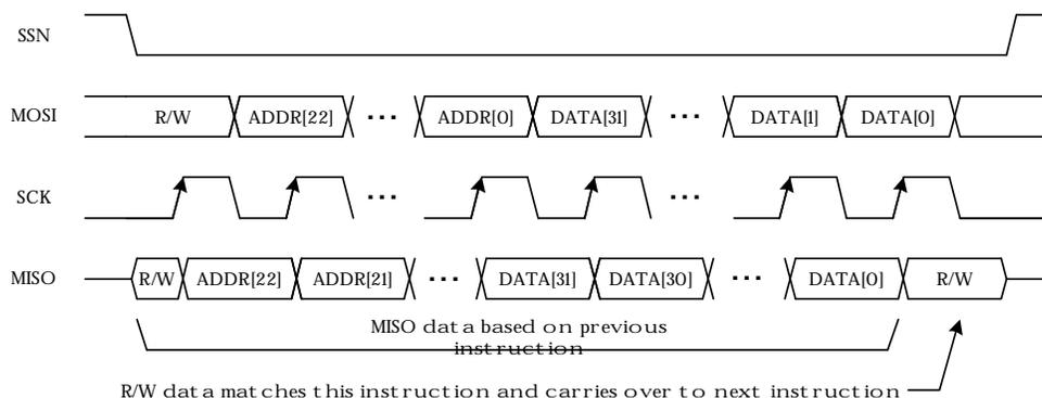
MISO output timing is the only difference between the two SPI modes. Sampling of MOSI on the rising SCK clock edge remains the same so writing to the VSC8258-01 device registers is identical in both modes. Thus the SPI\_CTRL.FAST\_MODE register setting may be modified using the SPI slave port to change the port's MISO output timing.
