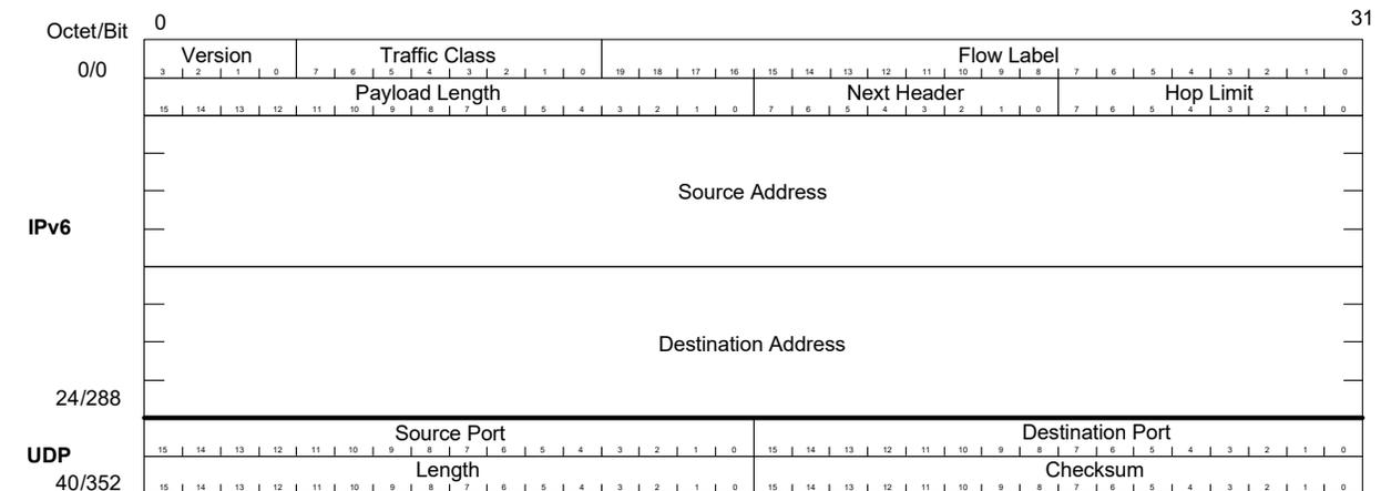
Per flow validation is performed on the Source or Destination Address in the IPv6 header. The comparator can be configured to indicate a match in the flow if the source, destination, or either the source or destination fields match.
