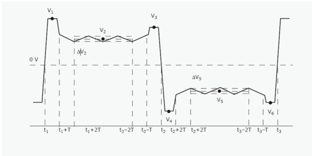
The output waveform is manipulated through the state of the coefficient  $C(-1)$ ,  $C(0)$ , and  $C(+1)$ .
