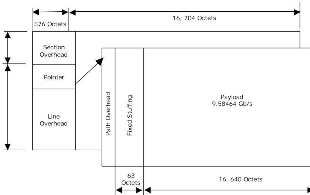
The following illustration shows the positions of the STS-192c/STM-64 section and line overhead octets within the WIS frame.
