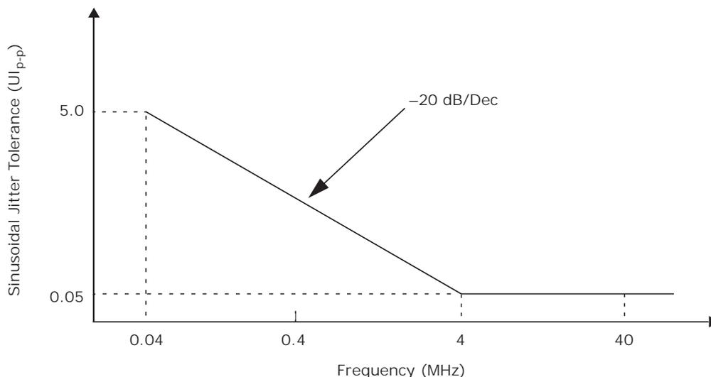
The following table lists the 10G input jitter specifications for the VSC8258-01 device.
