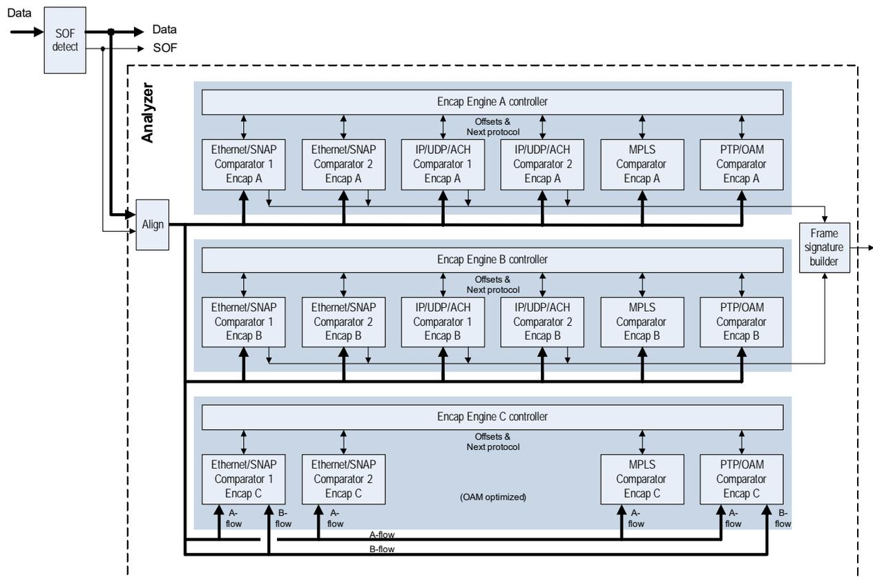
The analyzer process is divided into engines and stages. Each engine represents a particular encapsulation stack that must be matched. There are up to six stages in each engine. Each stage uses a comparator block that looks for a particular protocol. The comparison is performed stage-by-stage until the entire frame header has been parsed.
