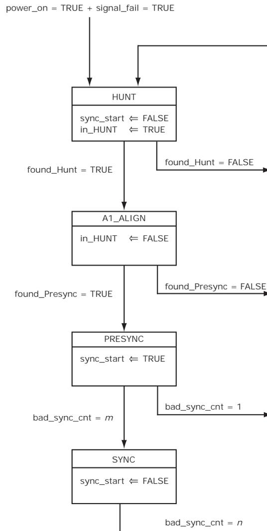
The following table lists the variables for the primary state diagram. The variables are reflected in registers (EWIS\_RX\_FRM\_CTRL1 and EWIS\_RX\_FRM\_CTRL2 that can be alternately reconfigured).
