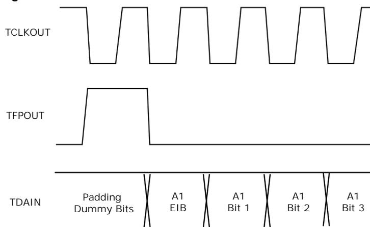
Some 9-bit words are error masks, such that the transmitted 9-bit word is the XOR of the TOSI 9-bit word and the pre-defined value within the chip if the EIB is enabled. This feature is best used for test purposes only.
