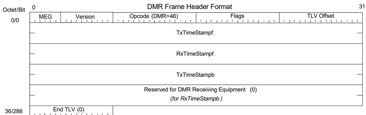
As with PTP, there is no protocol validation for Y.1731 frames; only interpretation of the header to determine what action to take. The first four bytes of the header are used to determine the action to be taken.
