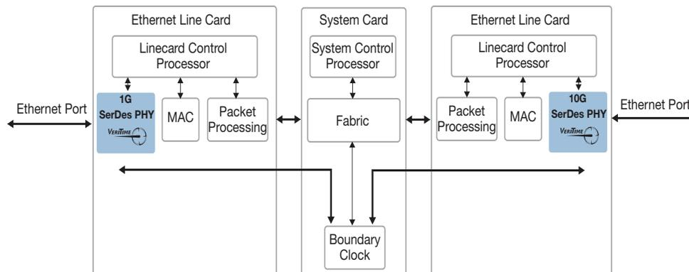
This solution also works for pizza boxes. To ensure that blade redundancy works, the PHYs for the redundant blades must have the same 1588-in-the-PHY configuration. Requirements for the rest of the system are:
