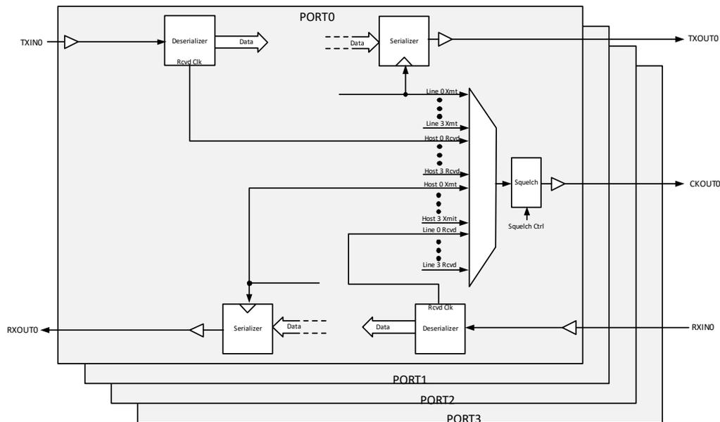
The rate of these clocks is the line rate divided by 32 or 64 (322.27 MHz or 161.13 MHz in 10G LAN mode, for example). There is no provision to synthesize a Sync-E-friendly rate on CKOUT[0:3]. However, should it be acceptable in a Sync-E application, the same clock squelching capability found on SCKOUT is available.
