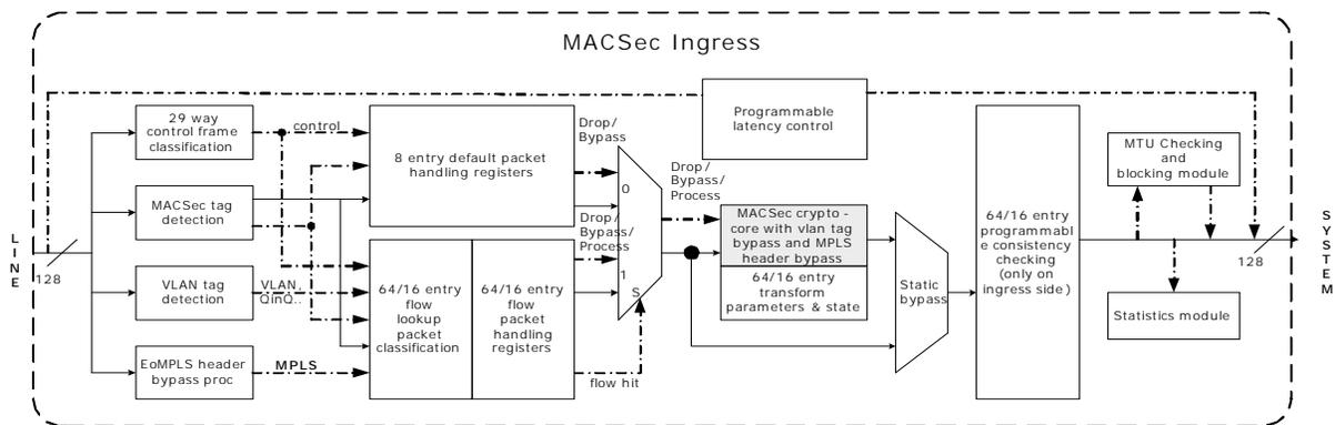
The following sections describe the pipeline stages. Of these pipeline stages, the MACsec transform stage is the only one that can modify the frame data or drop a frame completely (no frame will appear at the output of the pipeline in that case). Other stages can only perform the following actions for frame data:
