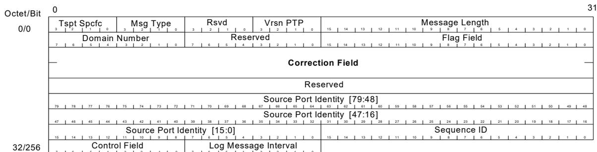
Unlike most of the other stages, there is no protocol validation for PTP frames; only interpretation of the header to determine what action to take. The first eight bytes of the header are used to determine the action to be taken. These match fields in the flow comparison registers with a corresponding set of command registers for each flow.
