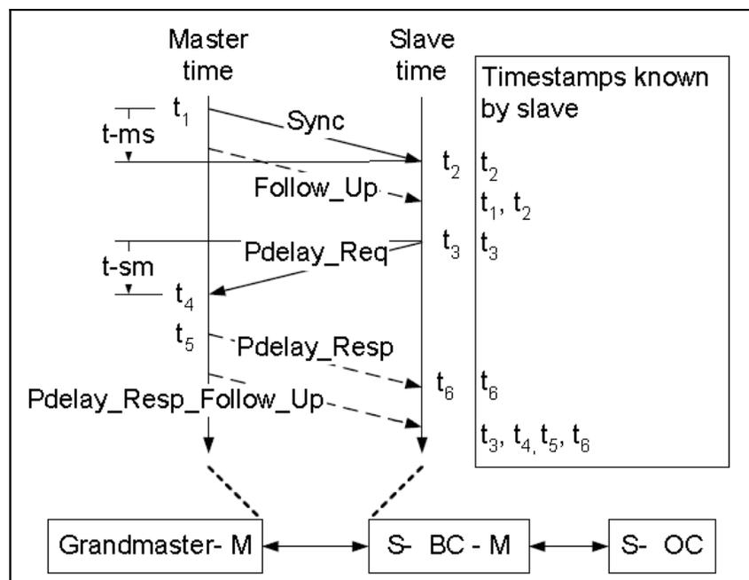
To calculate the path delays on a link, the IEEE 1588 engine (located somewhere in the system) generates Pdelay\_Req messages on all ports. When transmitted, the actual Tx time stamp t3 is saved for the CPU to read.
