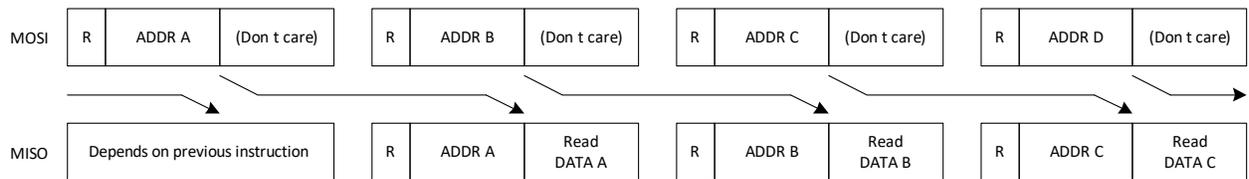
The SPI read instruction figures also point out the read/write state and address bits on the MISO output match the information received in the previous instruction. The SPI master could use this data to verify the device captured the previous instruction properly, or simply ignore the data. The following illustration shows the MISO output during write instructions reporting the previous instruction's read/write state, address, and register write data.
