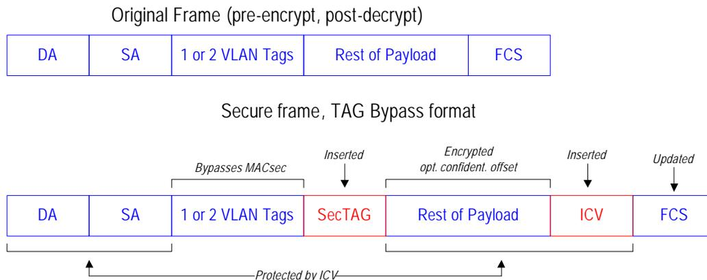
The following logic is used to process the tag bypass format.
