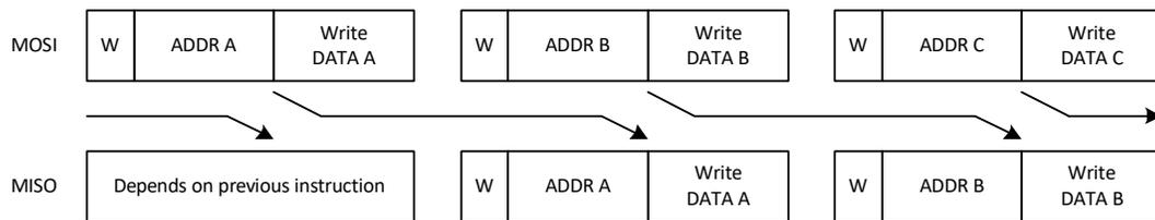
The following illustration shows that when a read instruction follows a write instruction, the MISO data during the read instruction is the data field from the previous write.
