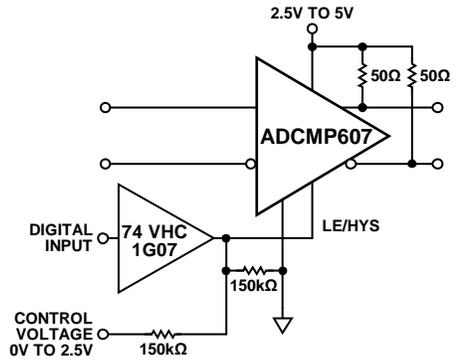
Figure 24. Hysteresis Adjustment with Latch on the ADCMP607
