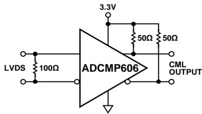
Figure 20. LVDS to CML on the ADCMP606
