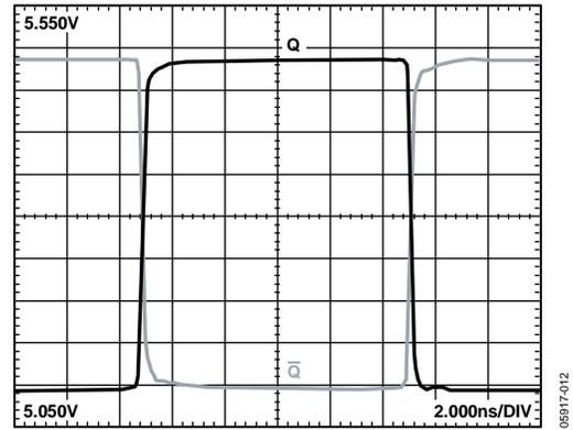
Figure 13. Output Waveform at  $V_{CC} = 5.5V$
