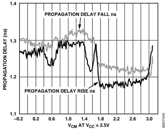
Figure 11. Propagation Delay vs. Input Common-Mode Voltage
