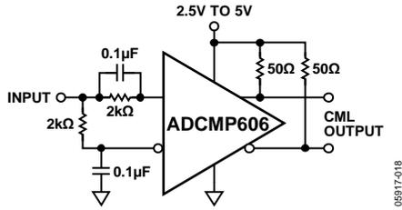
Figure 19. Self-Biased, 50% Slicer on the ADCMP606
