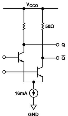
Figure 14. Simplified Schematic Diagram of CML-Compatible Output Stage
