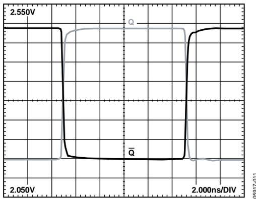
Figure 12. Output Waveform at  $V_{CC} = 2.5V$
