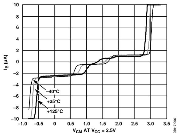
Figure 7. Input Bias Current vs. Input Common-Mode Voltage
