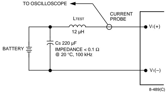
Note: Input reflected-ripple current is measured with a simulated source impedance ( $L_{TEST}$ ) of  $12\ \mu\text{H}$ . Capacitor  $C_s$  offsets possible battery impedance. Current is measured at the input of the module.
