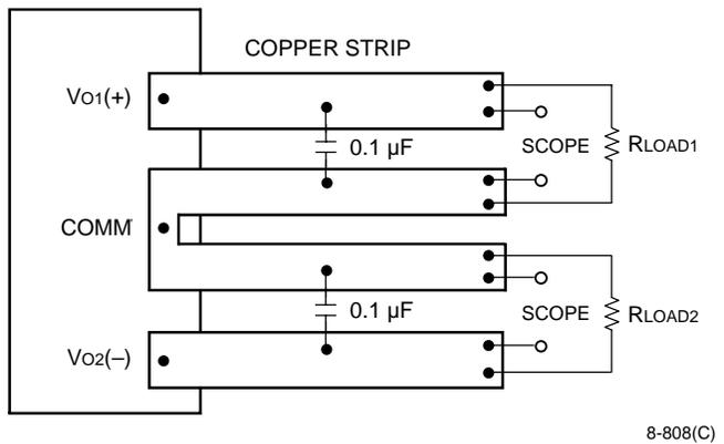
Note: Use a  $0.1\ \mu\text{F}$  ceramic capacitor. Scope measurement should be made using a BNC socket. Position the load between 50 mm (2 in.) and 75 mm (3 in.) from the module.
