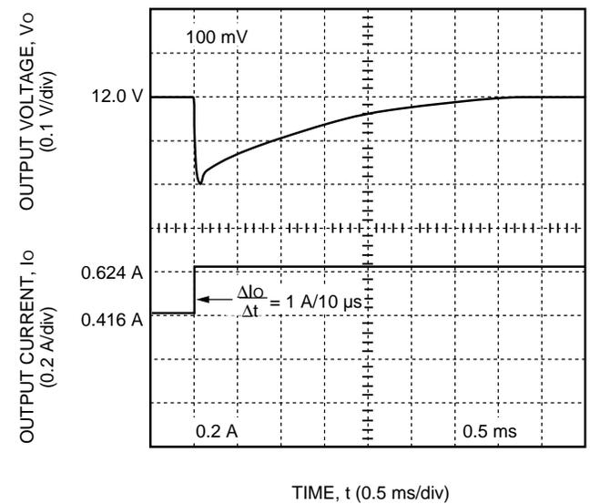
Figure 8. CW025 Dual Output-Series Typical 12 V Output Voltage Response to a Step Load Change from 50% to 75% of  $I_{o,max}$  at  $V_i = V_{i,nom}$  and  $T_c = 25\text{ }^\circ\text{C}$
