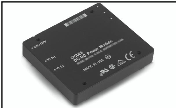
The CW025 Dual Output-Series Power Modules use advanced, surface-mount technology and deliver high-quality, compact, dc-dc conversion at an economical price.
