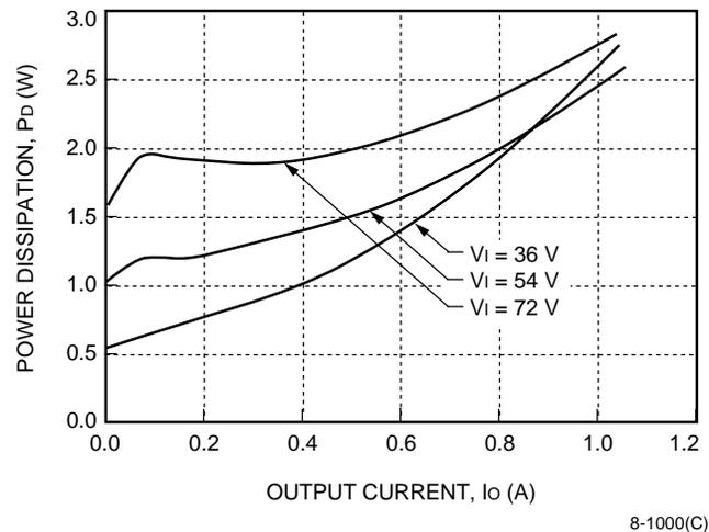
**Figure 17. 12 V Output Power Dissipation vs. Output Current**
