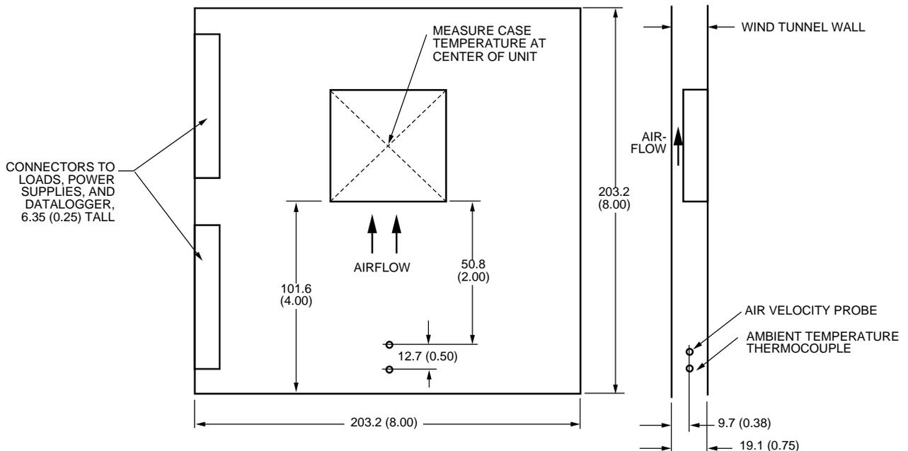
Note: Dimensions are in millimeters and (inches). Drawing is not to scale.
