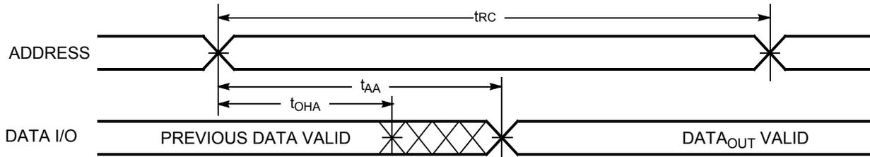
Figure 4. Read Cycle No. 2 ( $\overline{OE}$  Controlled) [20, 21]
