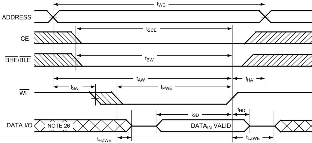
Figure 8. Write Cycle No. 4 ( $\overline{BHE}/\overline{BLE}$  Controlled,  $\overline{OE}$  LOW) <sup>[25]</sup>
