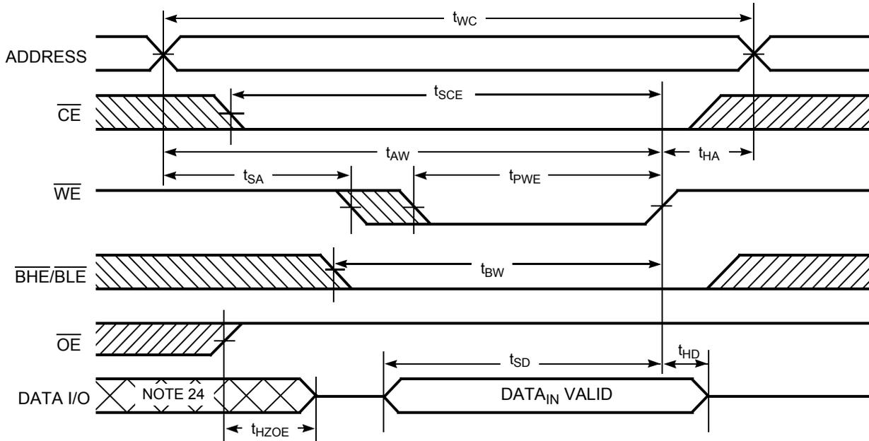
Figure 6. Write Cycle No. 2 ( $\overline{CE}$  Controlled) [22, 23]
