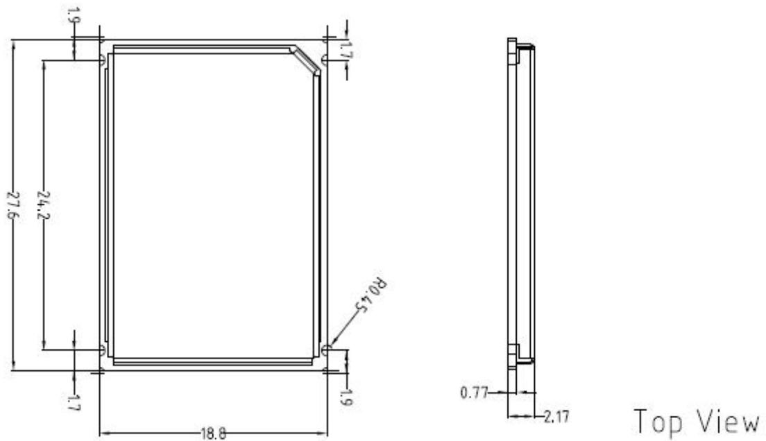
Figure 40: Dimensions of EMS31-US (all dimensions in mm)
