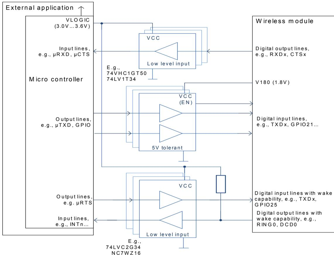
**Figure 26:** Sample level conversion circuit
