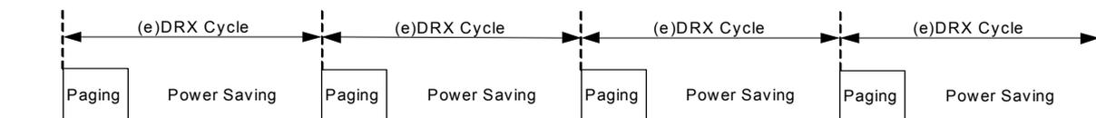
**Figure 33:** Power saving and paging in LTE networks in DRX and (e)DRX modes
