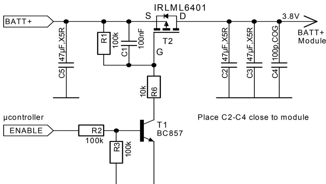
**Figure 27:** Simple circuit for applying power using an external  $\mu C$
