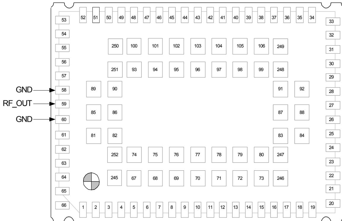
**Figure 16:** Antenna pad (bottom view)
