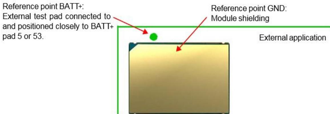
**Figure 36:** Position of reference points BATT+ and GND
