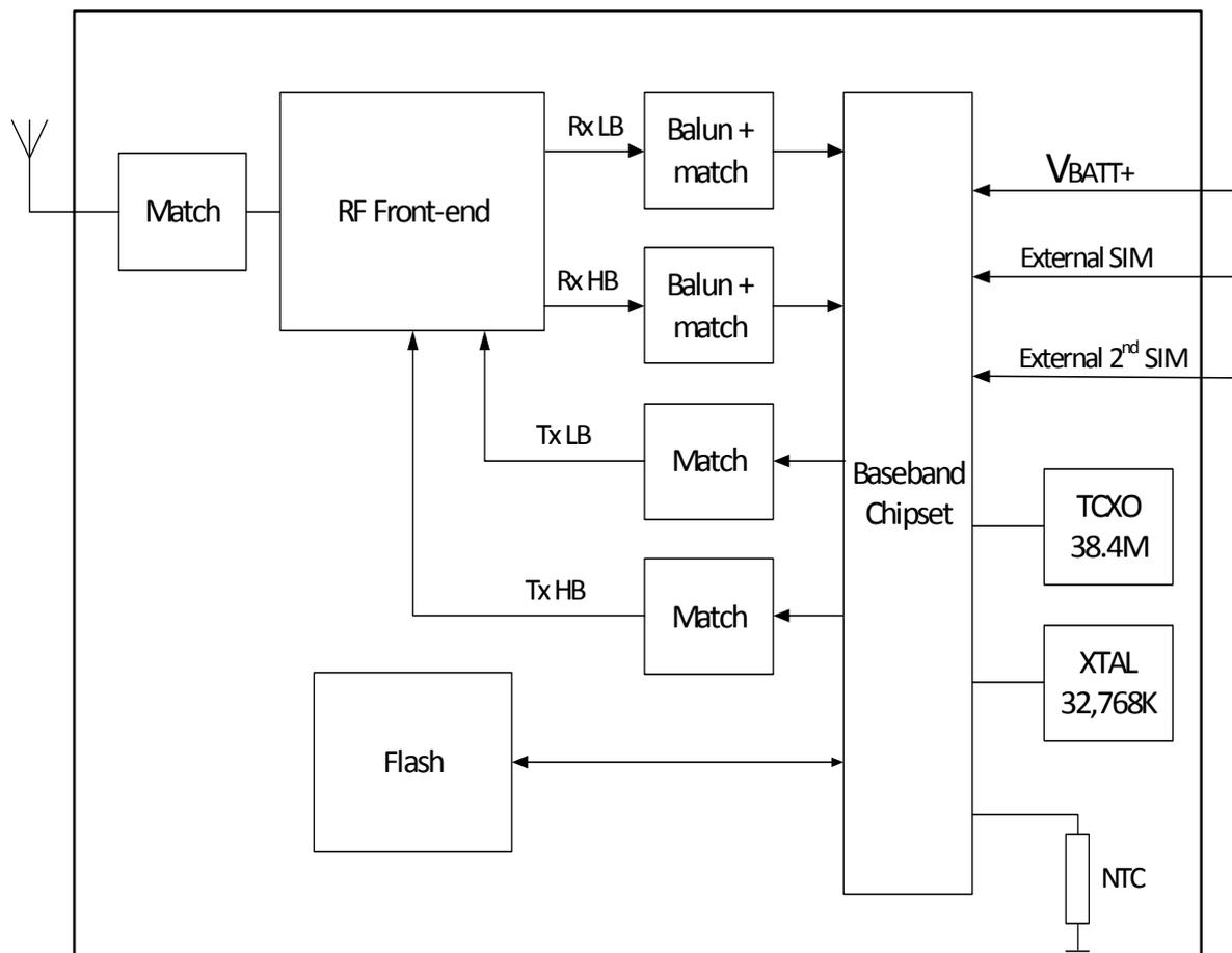
Figure 2: EMS31-US baseband block diagram
