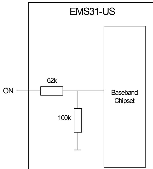
**Figure 28:** ON pin connection
