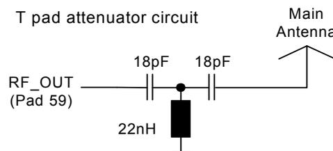
**Figure 37:** ESD protection for RF antenna interface
