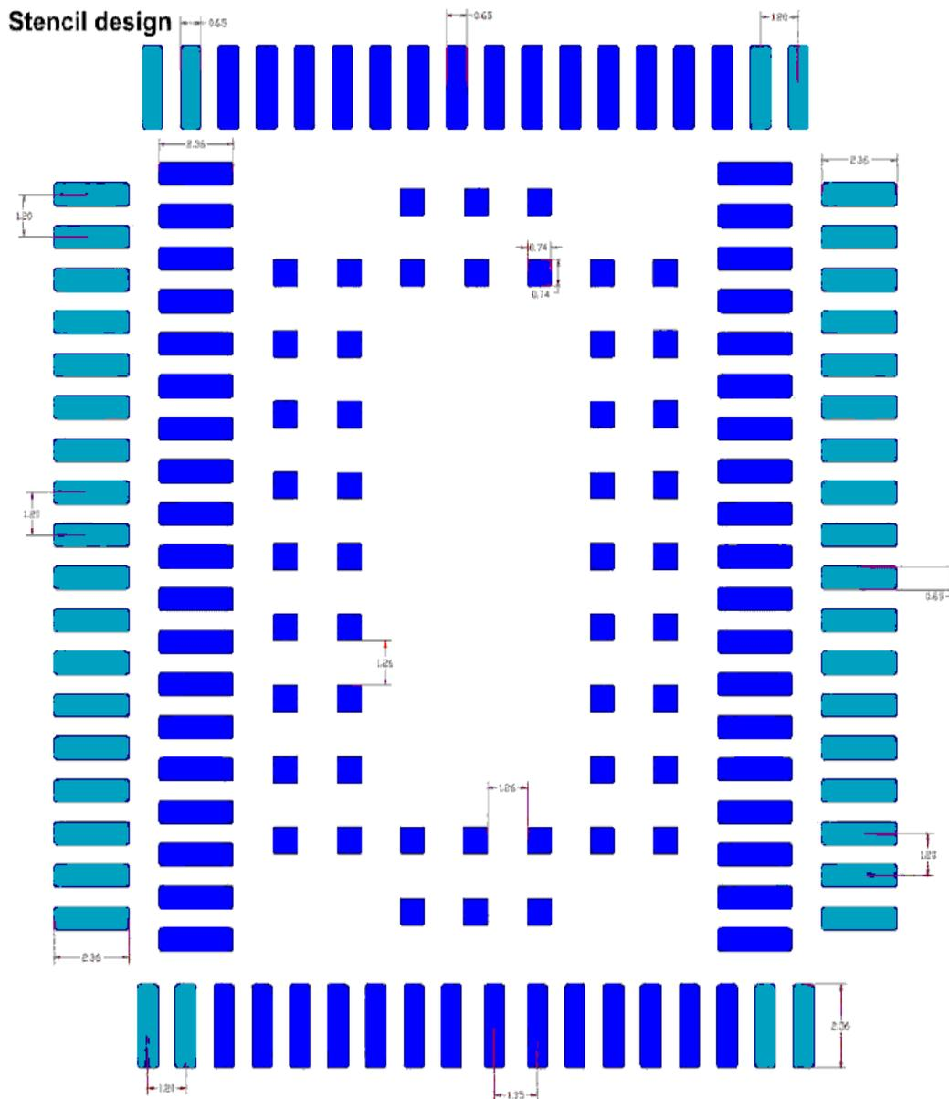
**Figure 43:** Recommended design for 150 micron thick stencil (top view, dual design)
