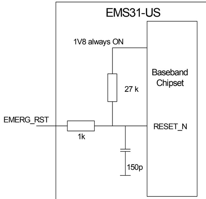
**Figure 30:** EMERG\_RST signal internal connection to chipset
