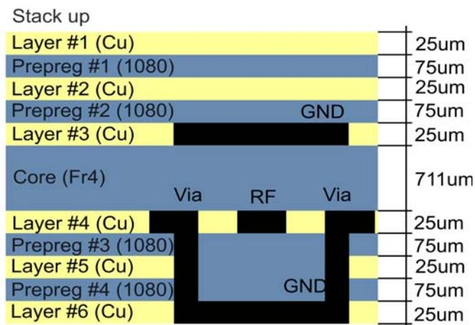
Figure 19: PCB layer stack of the EMS31-US evaluation board
