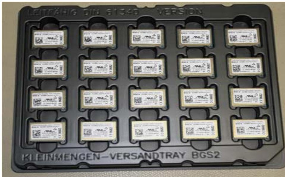
Figure 52: Tray to ship odd module amounts
