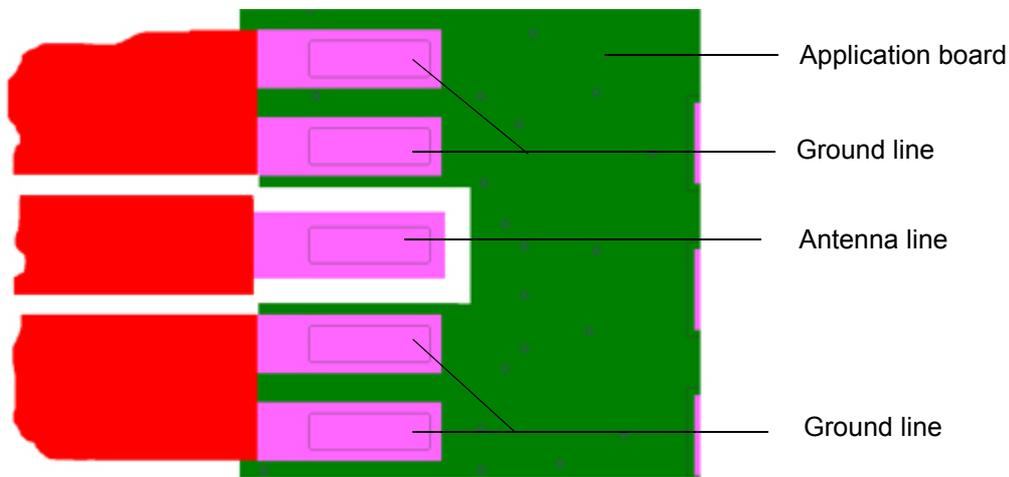
Figure 22: Microstrip line on 1.0mm Standard FR4 PCB - example 2
