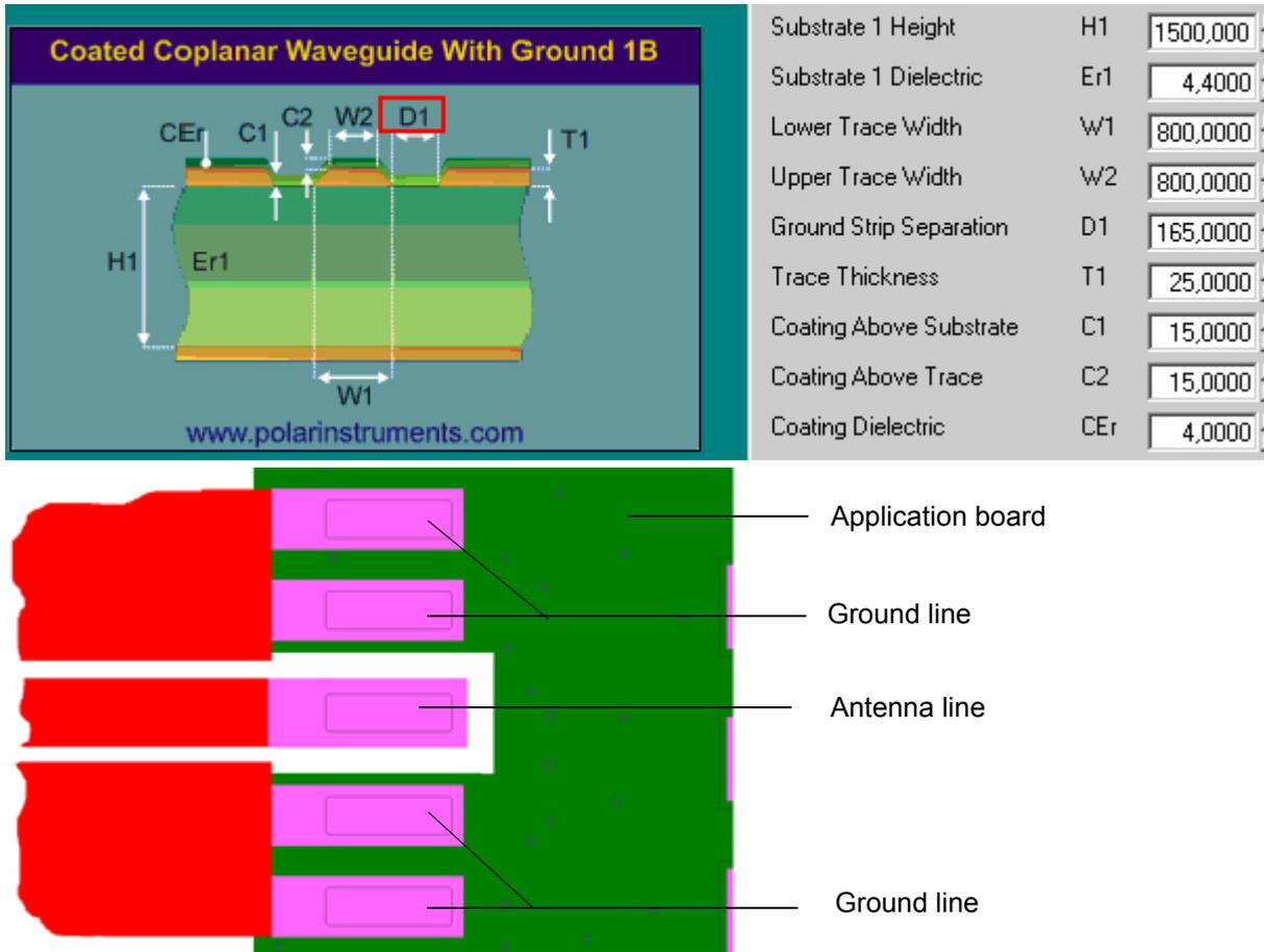
Figure 23: Microstrip line on 1.5mm Standard FR4 PCB - example 1
