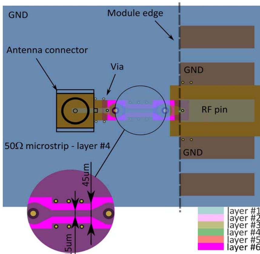
Figure 18: Routing to application's RF connector - Top view
