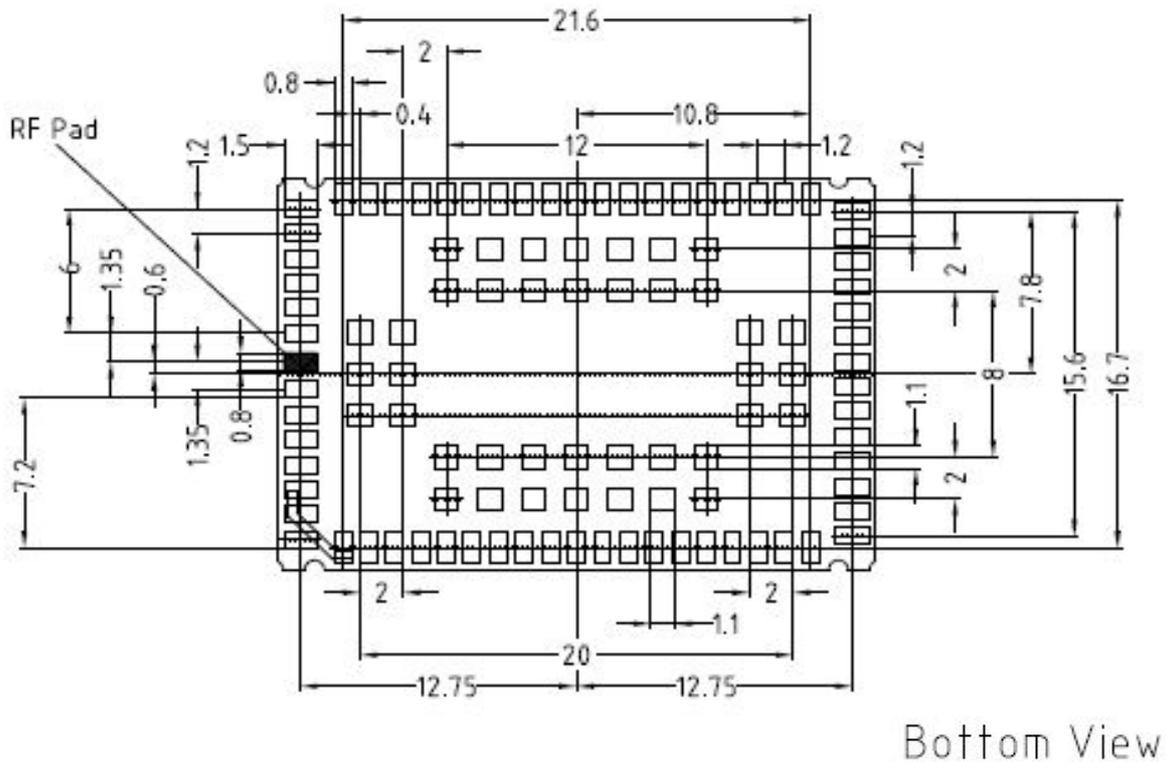
Figure 41: Dimensions of EMS31-US (all dimensions in mm) - bottom view
