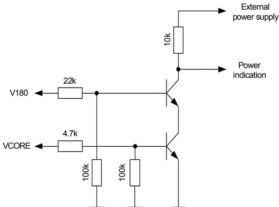
Figure 13: Power indication circuit
