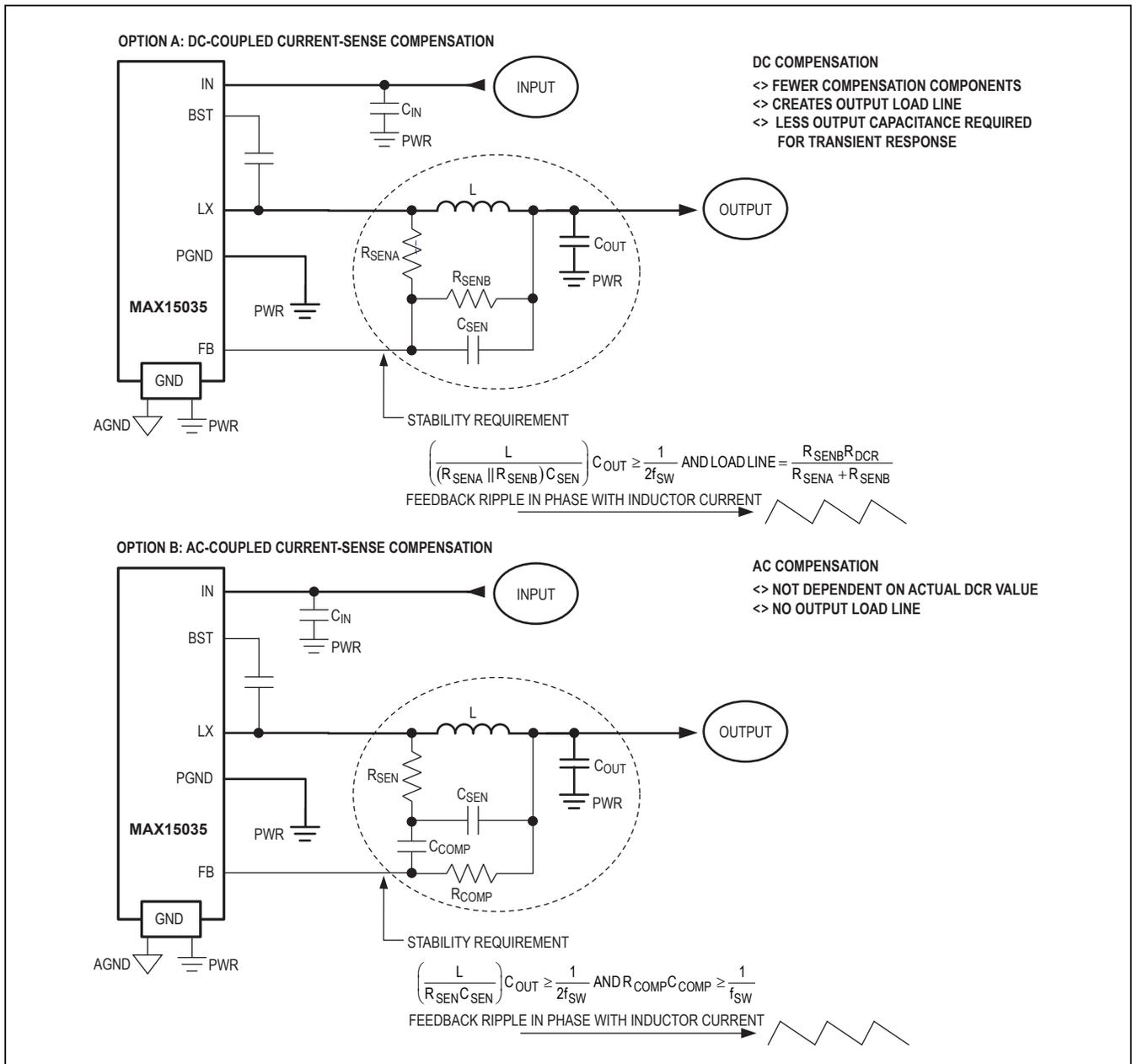
Figure 11. Feedback Compensation for Ceramic Output Capacitors
