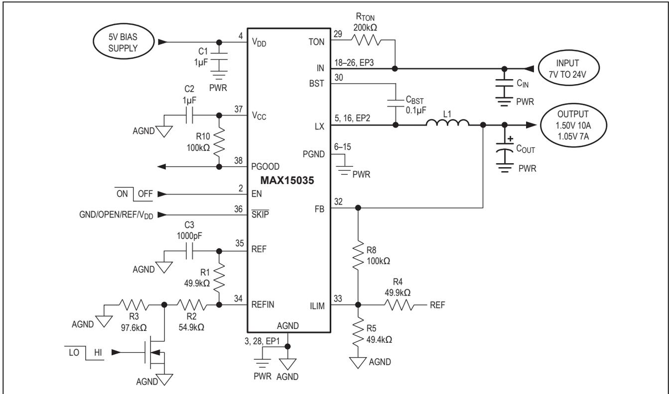
Figure 8. Standard Application with Foldback Current-Limit Protection
