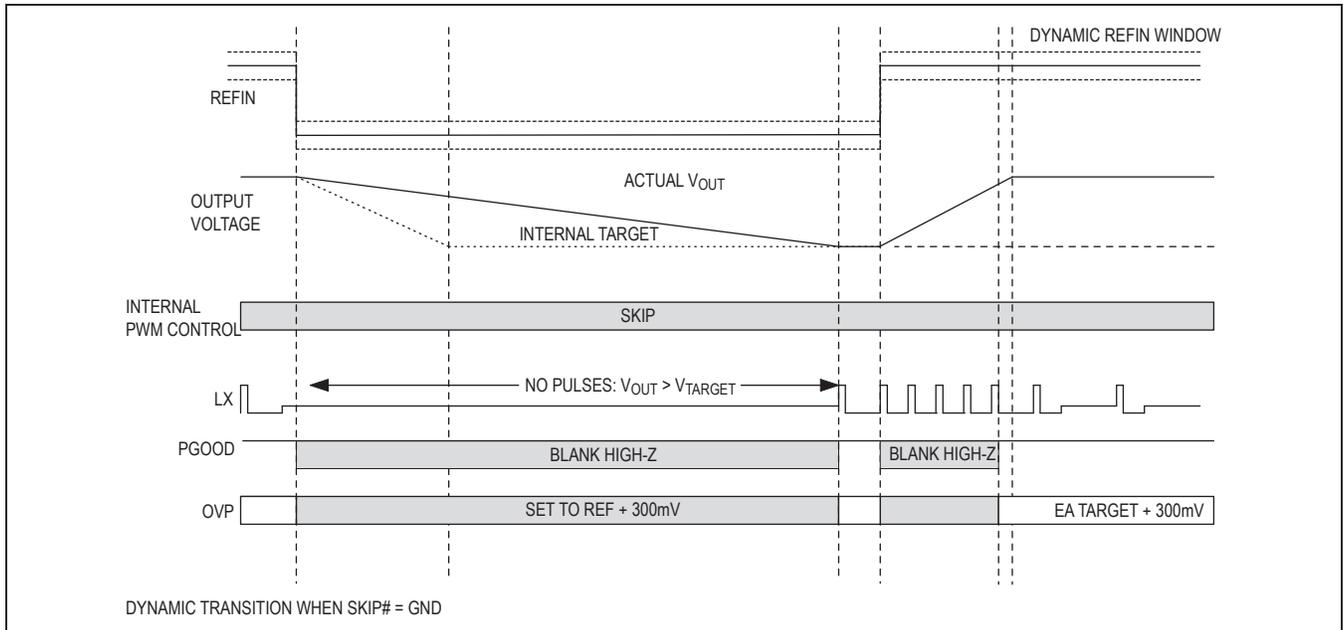
Figure 4. Dynamic Transition when  $\overline{SKIP} = GND$
