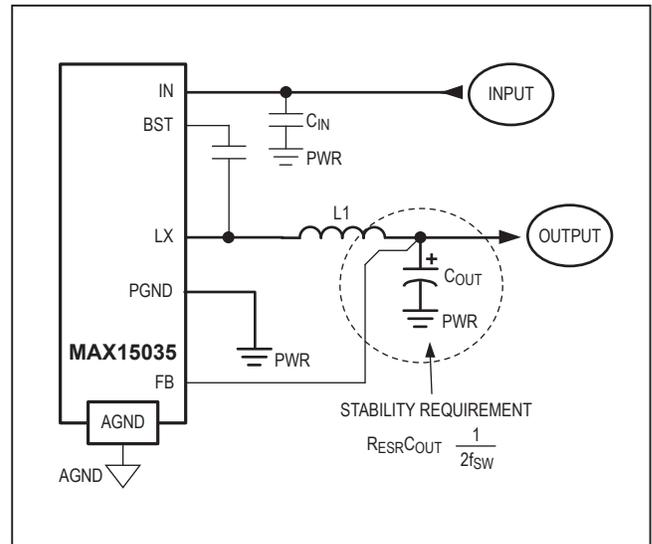
Figure 9. Standard Application with Output Polymer or Tantalum
