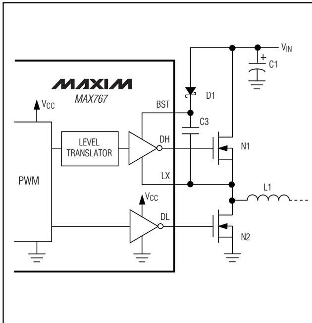
Figure 4. Boost Supply for High-Side Gate Driver
