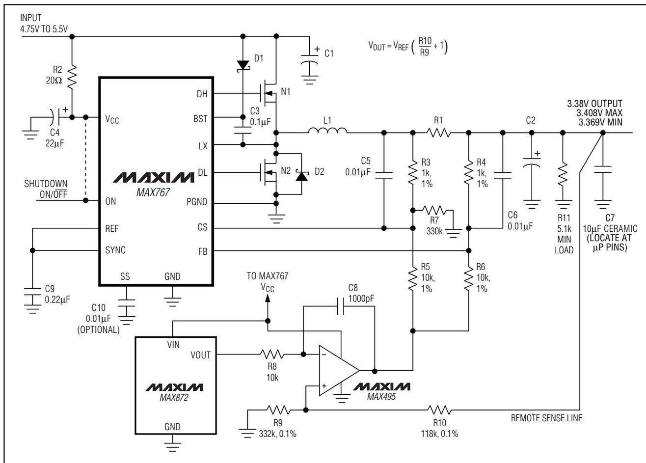
Figure 6. High-Accuracy CPU Power Supply with External Reference
