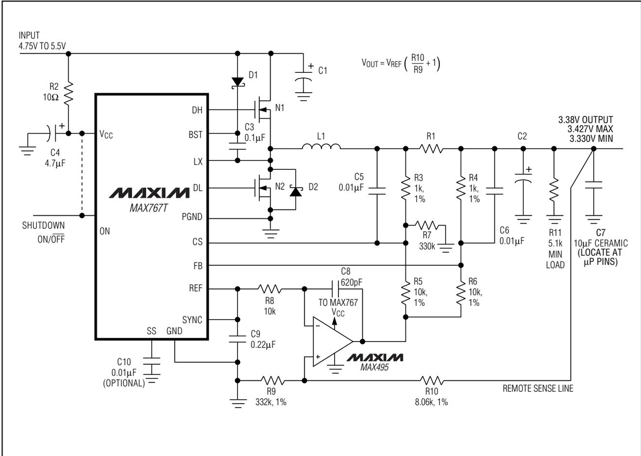
Figure 5. High-Accuracy CPU Power Supply with Internal Reference
