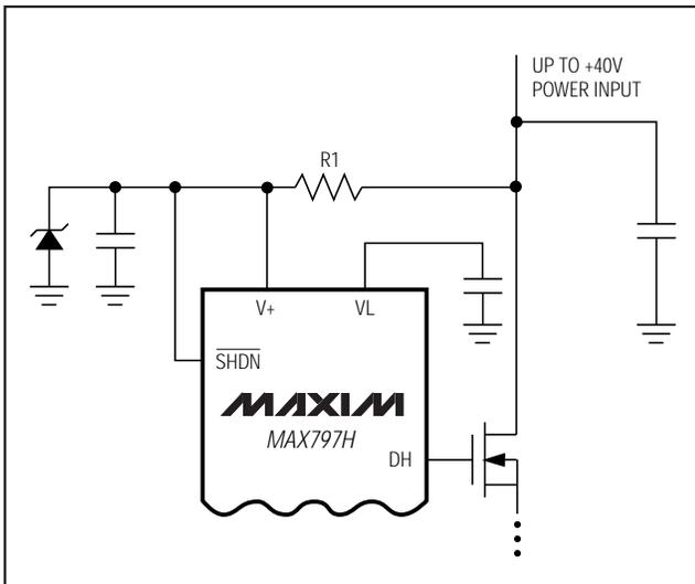
Figure 4. Powering V+ with a Zener Shunt Regulator
