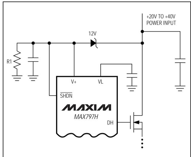
Figure 5. Powering V+ with a Zener Dropping Diode
