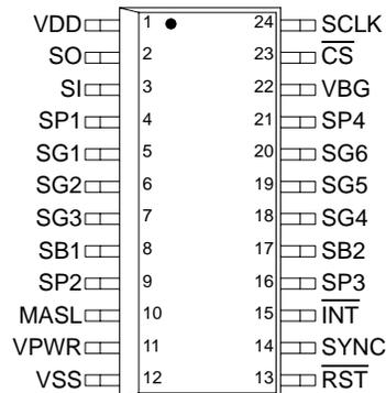
Figure 3. 33884 Pin Connections
