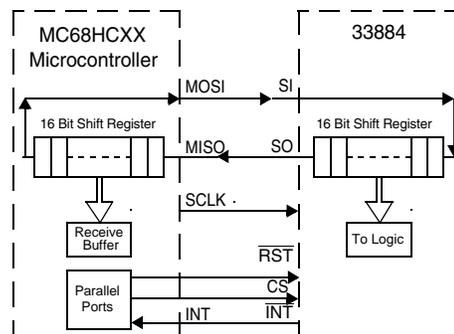
**Figure 4. SPI Interface with Microprocessor**
