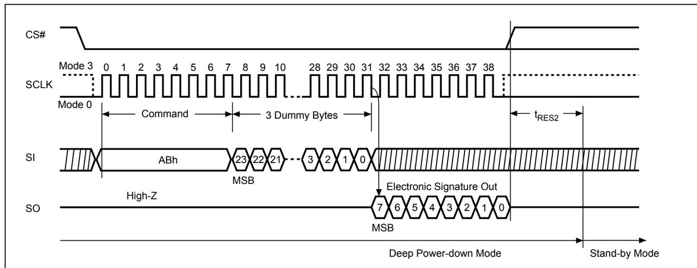
**Figure 28. Release from Deep Power-down (RDP) Sequence**
