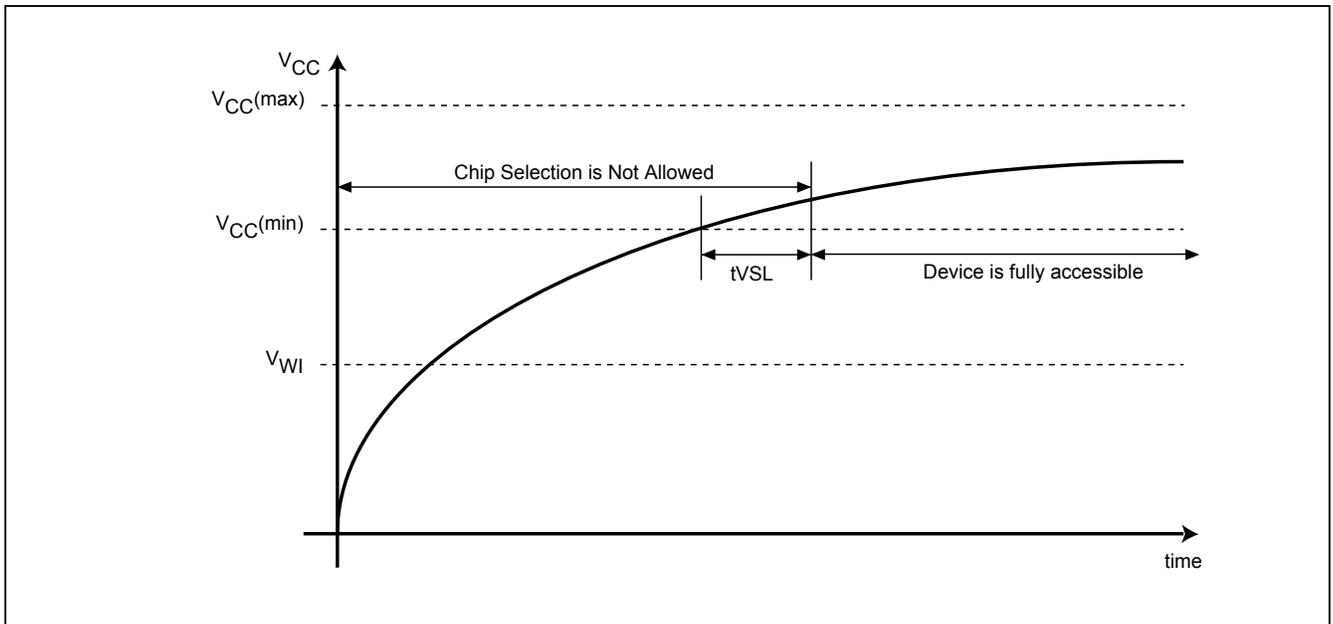
**Figure 50. Power Up/Down and Voltage Drop**
