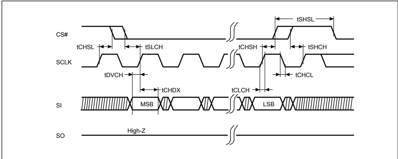
**Figure 44. Output Timing**
