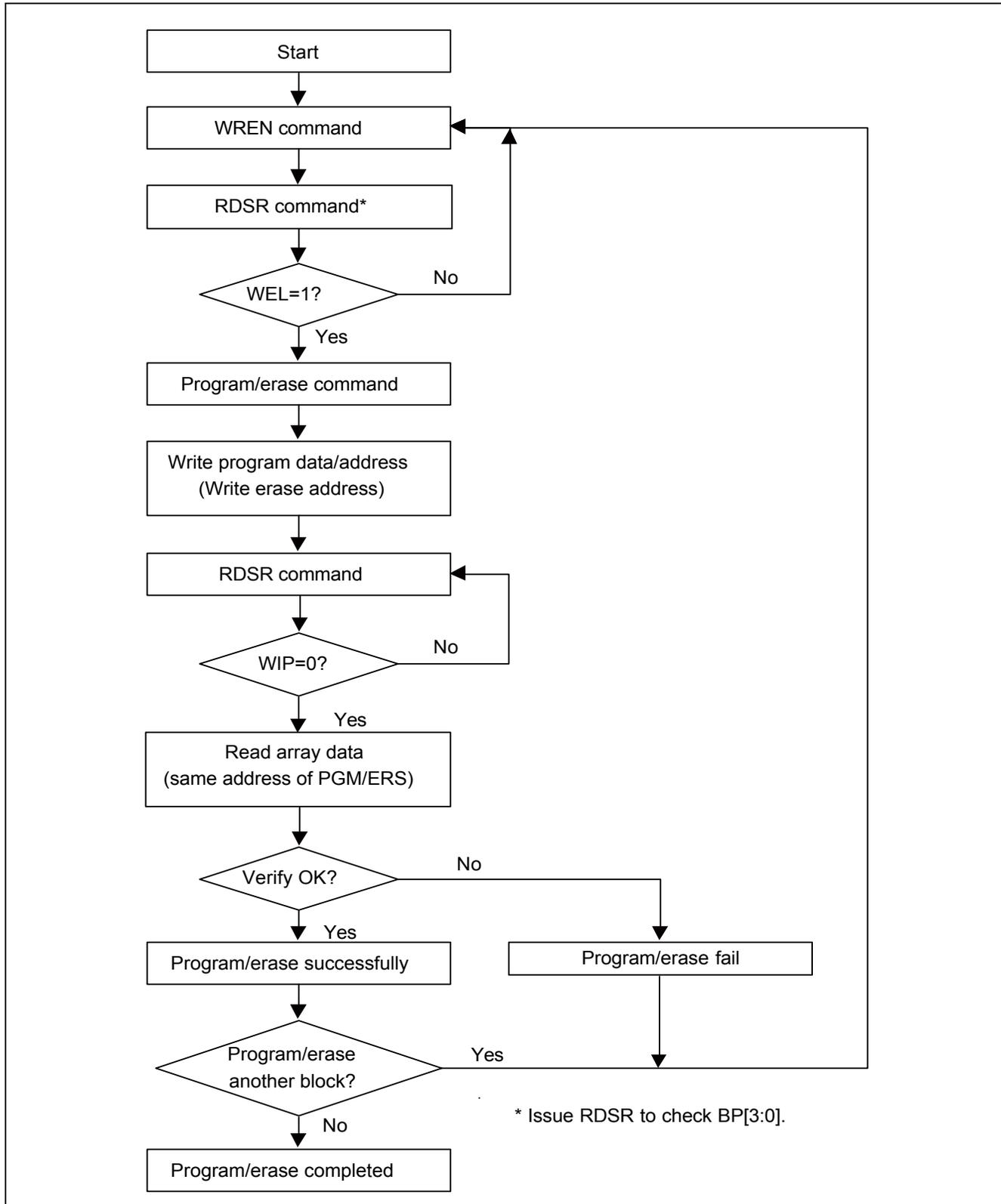
**Figure 25. Program/Erase Flow(2) without read array data**
