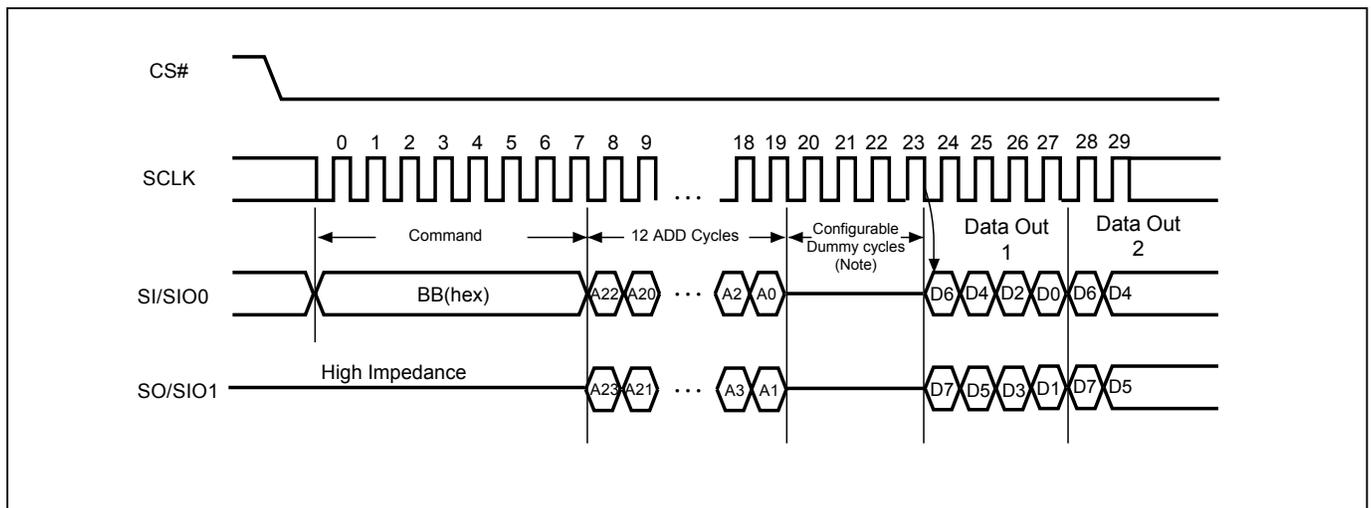
Note: The Configurable Dummy Cycle is set by Configuration Register Bit. Please refer to ["Table 7. Dummy Cycle and Frequency Table"](#).
