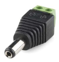
**Description:** This adapter allows you to connect a barrel jack connector to bare wires. One end has screw terminals and the other has a 5.5x2.1mm, center-positive male barrel jack. If you need to connect bare wires to a barrel jack on an Arduino or a development board, this might be the simple solution.
