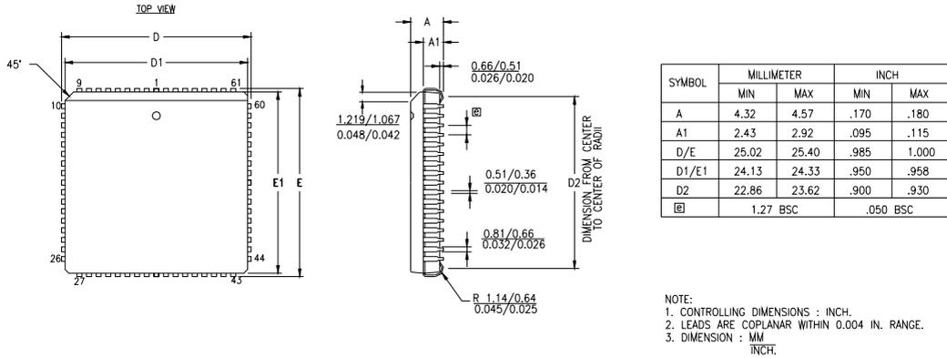
Figure 107. 68-Lead Plastic Lead Chip Carrier Package (PLCC)
