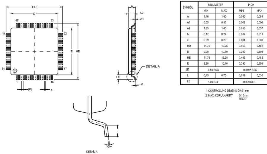
Figure 106. 64-Lead Low-Profile Quad Flat Package (LQFP)
