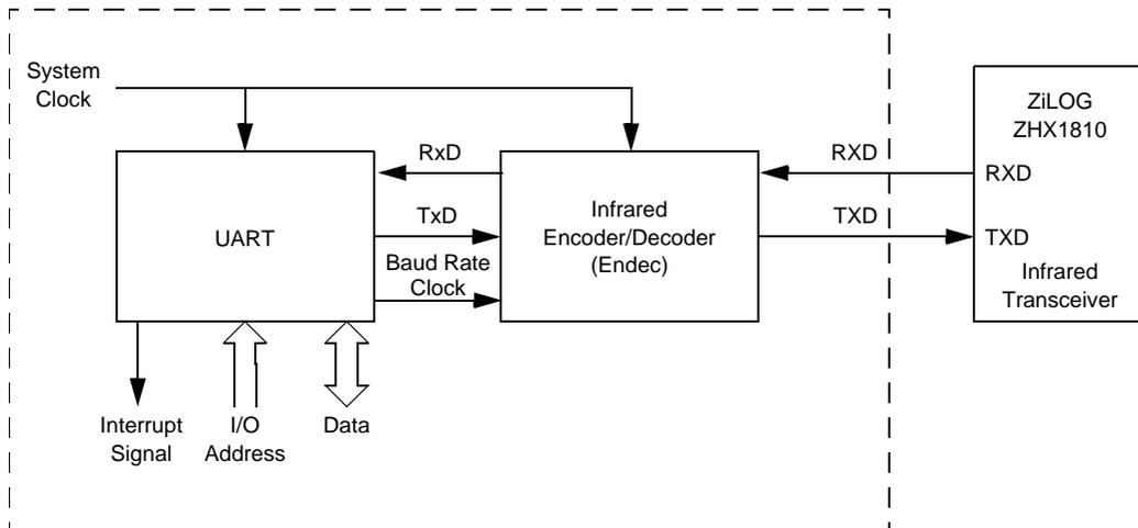
Figure 71. Infrared Data Communication System Block Diagram
