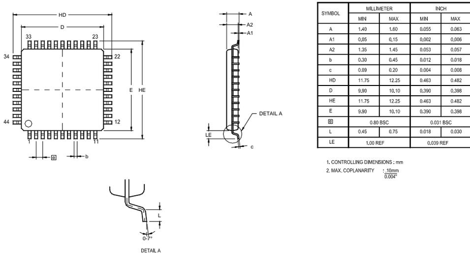
Figure 104. 44-Lead Low-Profile Quad Flat Package (LQFP)
