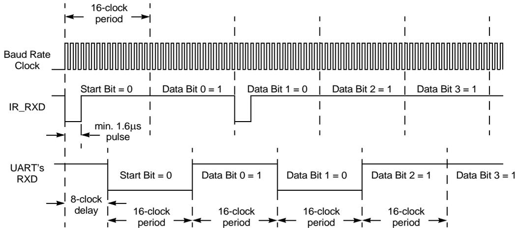
Figure 73. Infrared Data Reception
