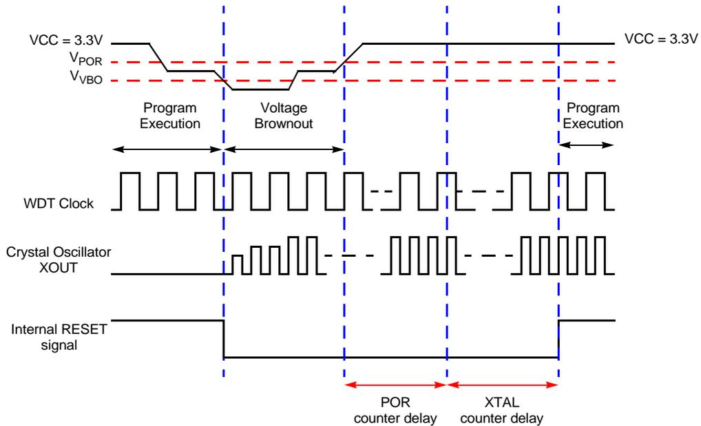
Figure 63. Voltage Brown-Out Reset Operation (not to scale)
