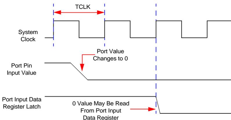
**Figure 93. Port Input Sample Timing**
