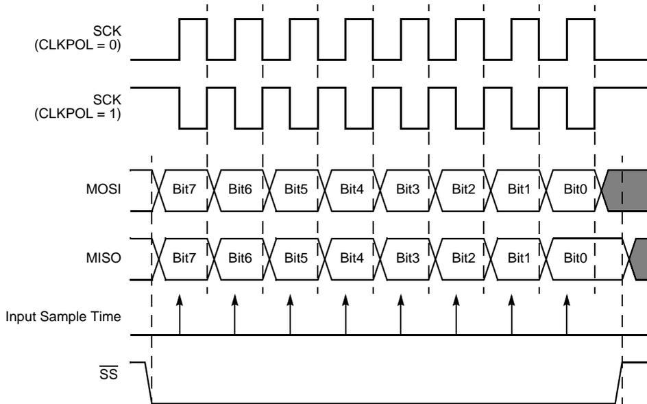
**Figure 77. SPI Timing When PHASE is 0**
