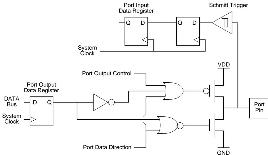
**Figure 64. GPIO Port Pin Block Diagram**
