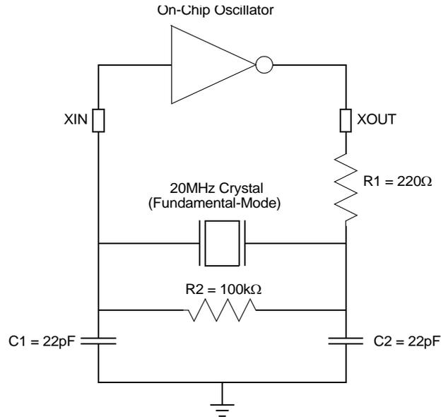
**Figure 90. Recommended Crystal Oscillator Configuration (20MHz operation)**
