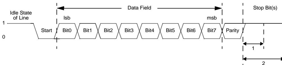
**Figure 69. UART Asynchronous Data Format with Parity**
