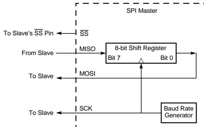
Figure 74. SPI Configured as a Master in a Single Master, Single Slave System
