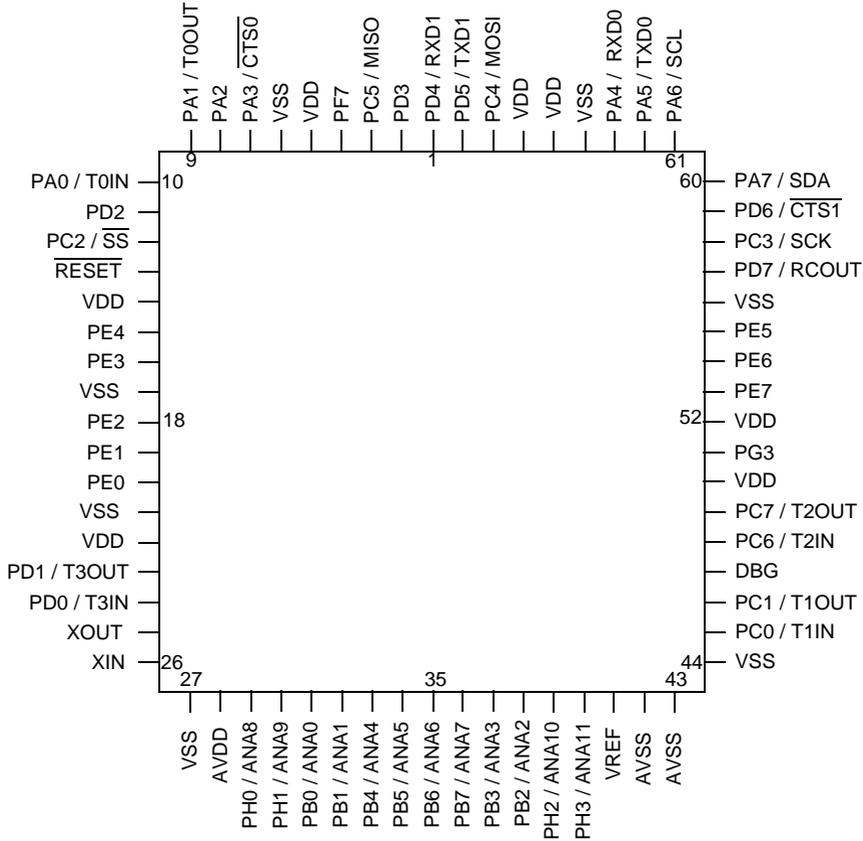
Figure 60. Z8Fxx02 in 68-Pin Plastic Leaded Chip Carrier (PLCC)
