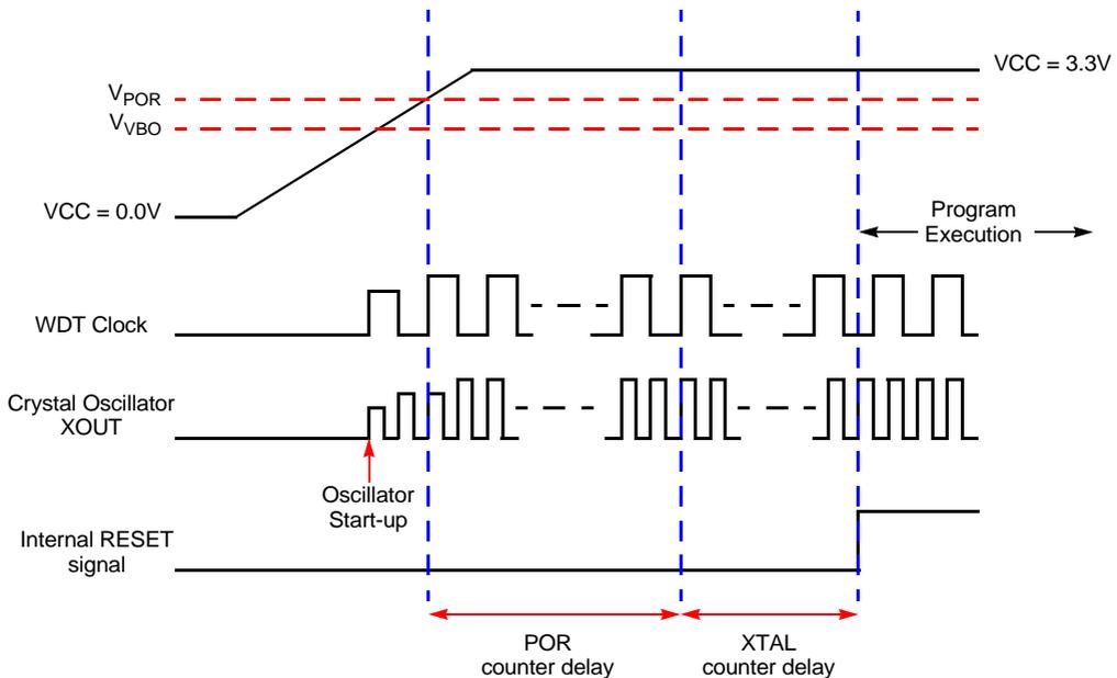
Figure 62. Power-On Reset Operation (not to scale)
