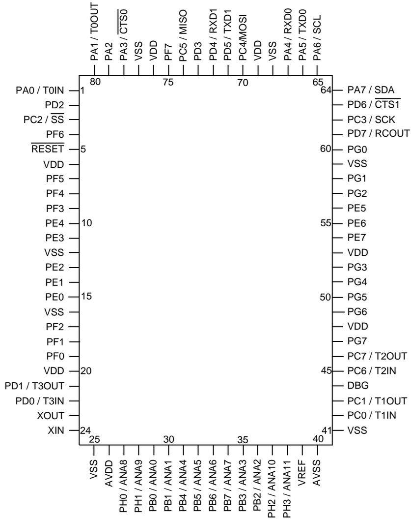
Figure 61. Z8Fxx03 in 80-Pin Quad Flat Package (QFP)
