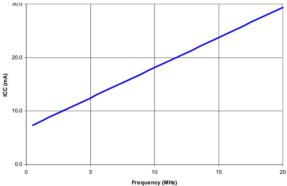
**Figure 91. Nominal ICC Versus System Clock Frequency**
