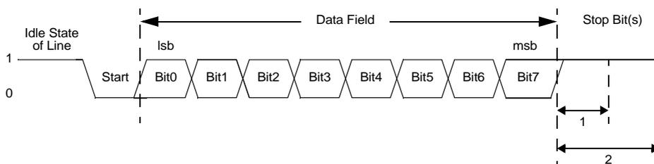
**Figure 68. UART Asynchronous Data Format without Parity**
