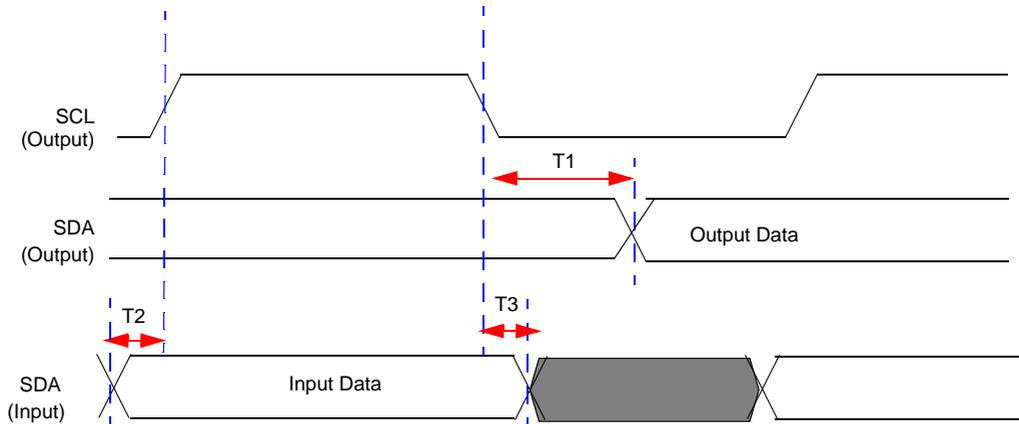
Figure 98. I<sup>2</sup>C Timing
