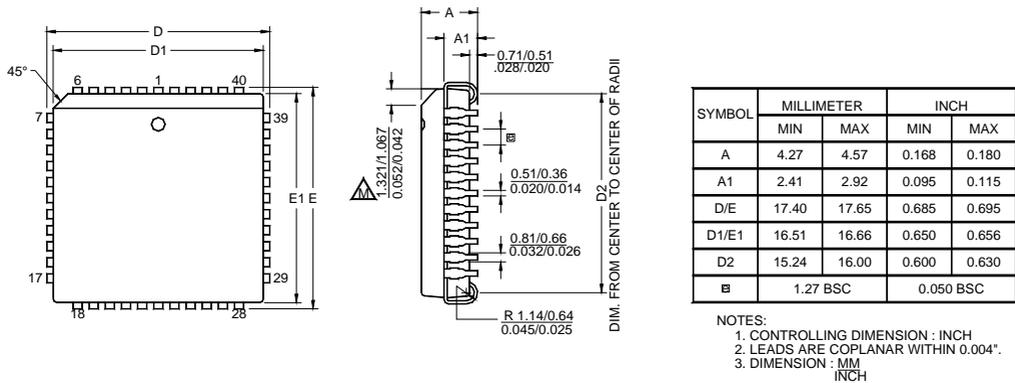
Figure 105. 44-Lead Plastic Lead Chip Carrier Package (PLCC)
