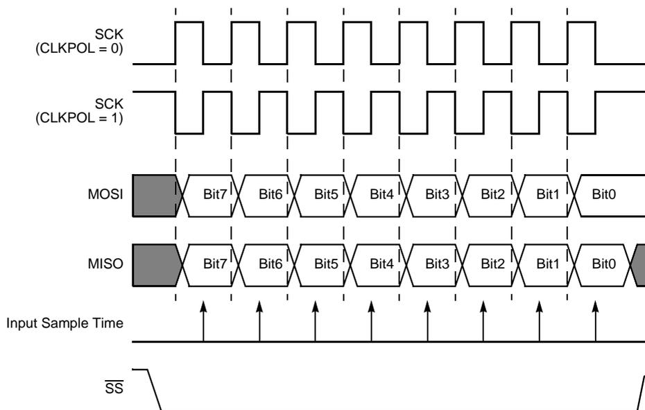
Figure 78. SPI Timing When PHASE is 1
