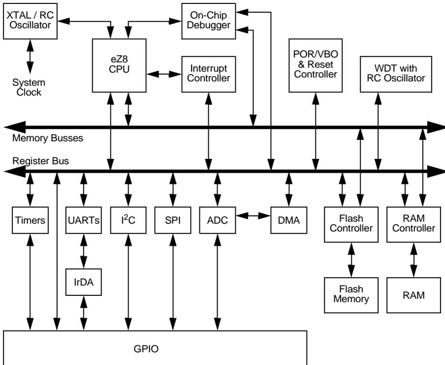
Figure 55. Z8 Encore!<sup>®</sup> Block Diagram
