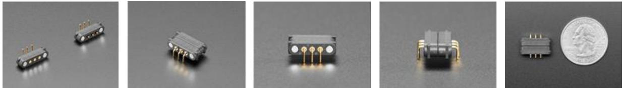
If you love power adapters or toys & gadgets that have magnetic connections, you can now experiment with these futuristic connectors easily. It's sorta like a DIY "MagSafe-styled" connector, with three 0.1" spaced contact pogo pins and a right angle solderable connection to your PCB. If you've ever owned a MacBook or a littleBits set, you'll find the functionality familiar.
