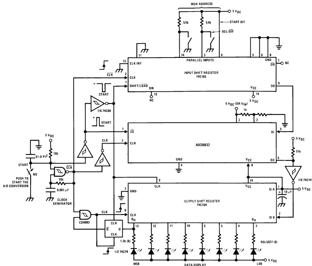
Figure 30. A “Stand-Alone” Hook-Up for ADC08832 Evaluation
