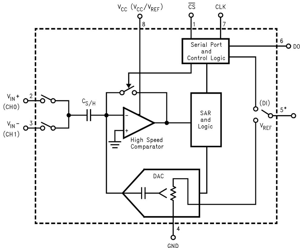
\*For ADC08831  $V_{REF}$  pin is available, for ADC08832 DI pin is available, and  $V_{REF}$  is tied to  $V_{CC}$
