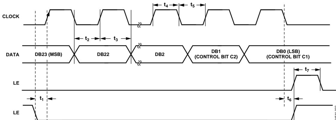
Figure 2. Timing Diagram
