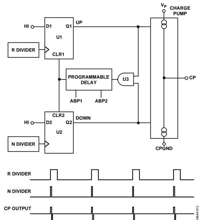
Figure 12. PFD Simplified Schematic and Timing (In Lock)
