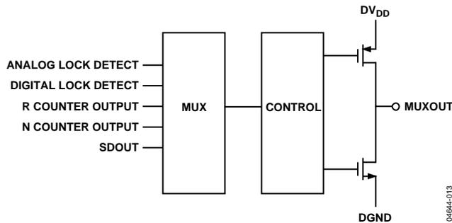
Figure 13. MUXOUT Circuit
