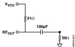
Figure 20. Simple ADF4360-0 Output Stage
