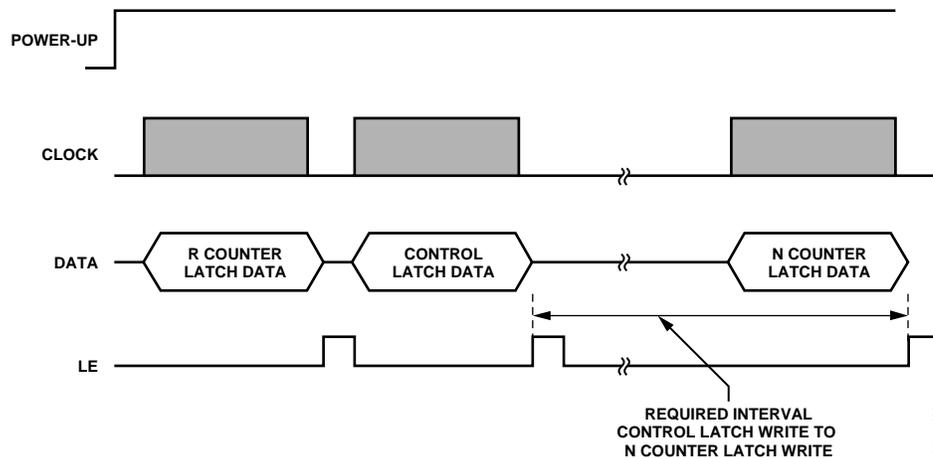
Figure 16. ADF4360-0 Power-Up Timing
