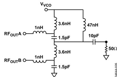
Figure 22. Balun for Combining ADF4360-0 RF Outputs
