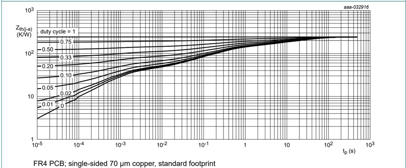
FR4 PCB; single-sided 70  $\mu\text{m}$  copper, standard footprint
