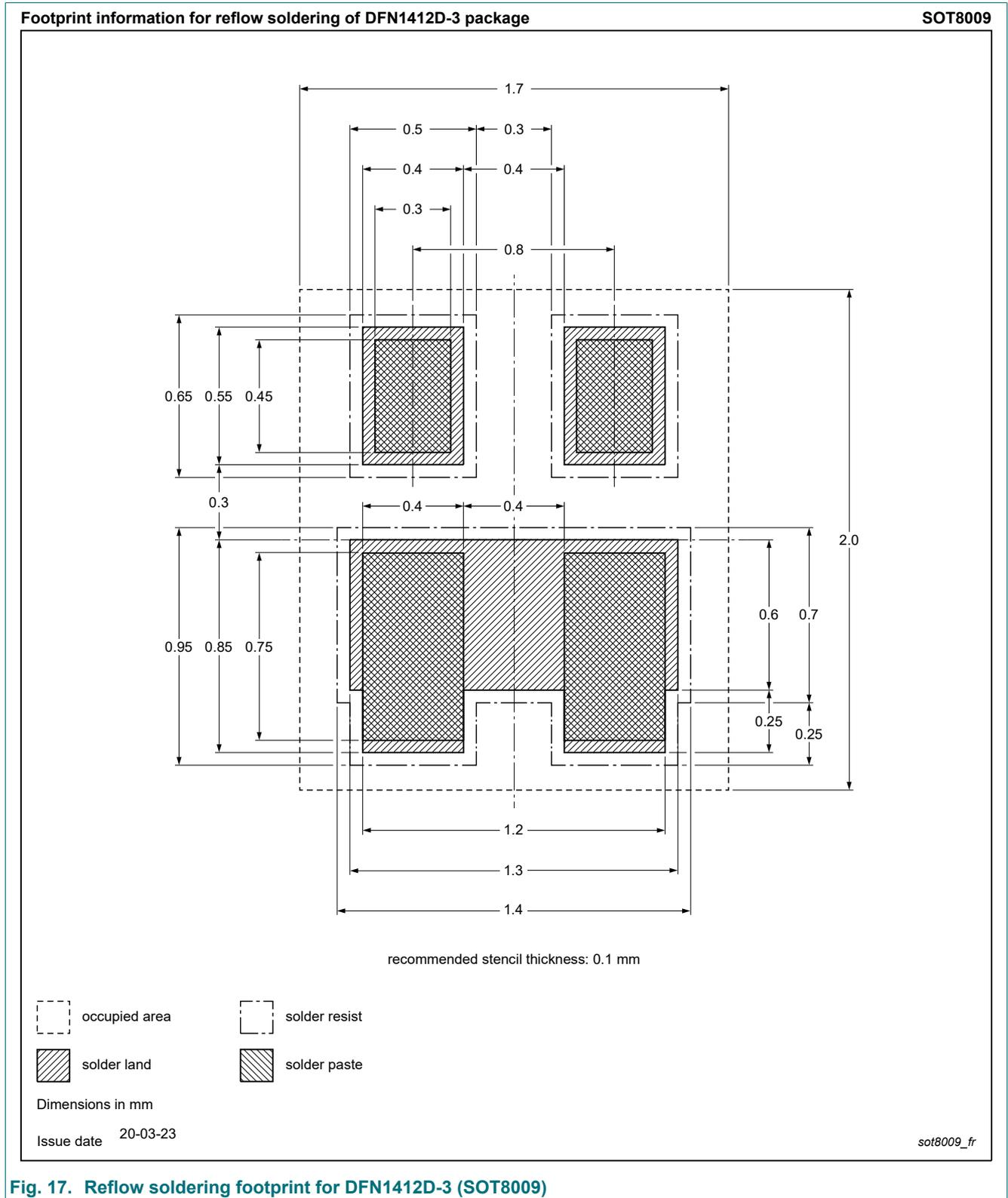
**Fig. 17. Reflow soldering footprint for DFN1412D-3 (SOT8009)**
