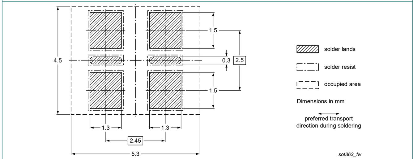
Fig. 12. Wave soldering footprint for TSSOP6 (SOT363)
