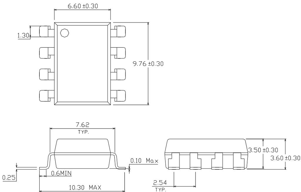
**8 PIN DIP HIGH SPEED 1Mbit/s TRANSISTOR
