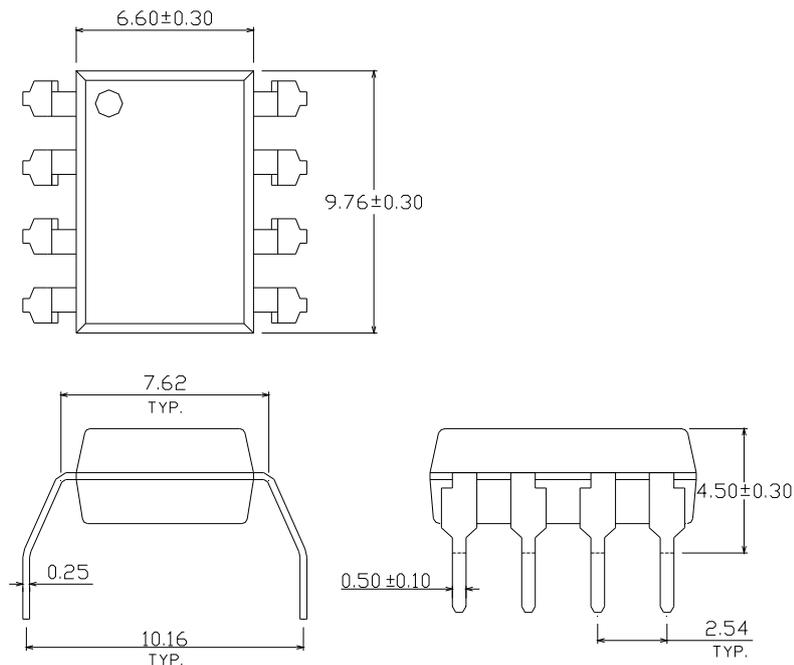
**8 PIN DIP HIGH SPEED 1Mbit/s TRANSISTOR
