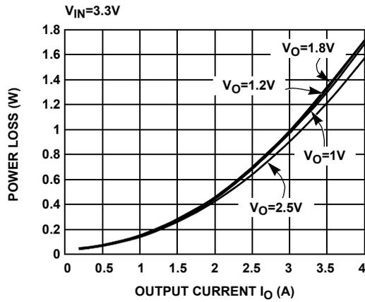
FIGURE 3. EL7563CM CONVERTER POWER LOSS vs I<sub>O</sub>
