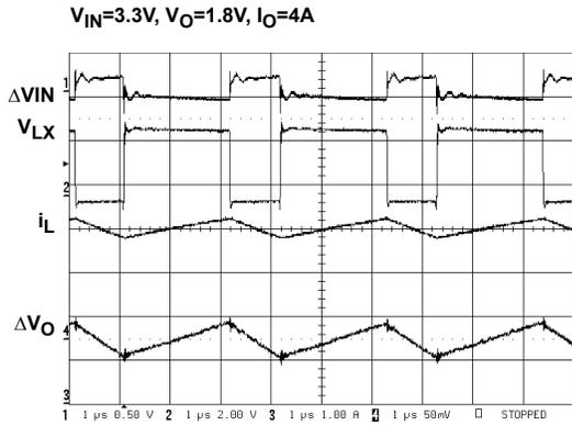
FIGURE 15. SWITCHING WAVEFORMS
