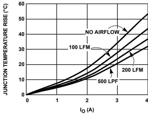
FIGURE 9. EL7563CM JUNCTION TEMPERATURE RISE ON DEMO BOARD
