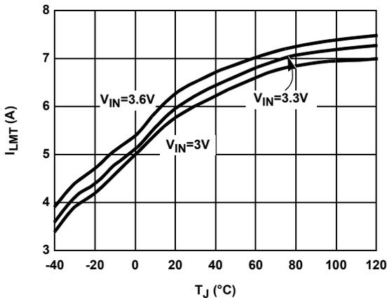
FIGURE 13. CURRENT LIMIT vs T<sub>J</sub>
