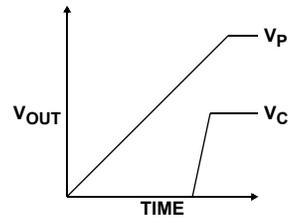
The second way of offset tracking is to use the EN and Power Good pins, as shown in Figure 25. In this configuration,  $V_P$  does not have to be larger than  $V_C$ .
