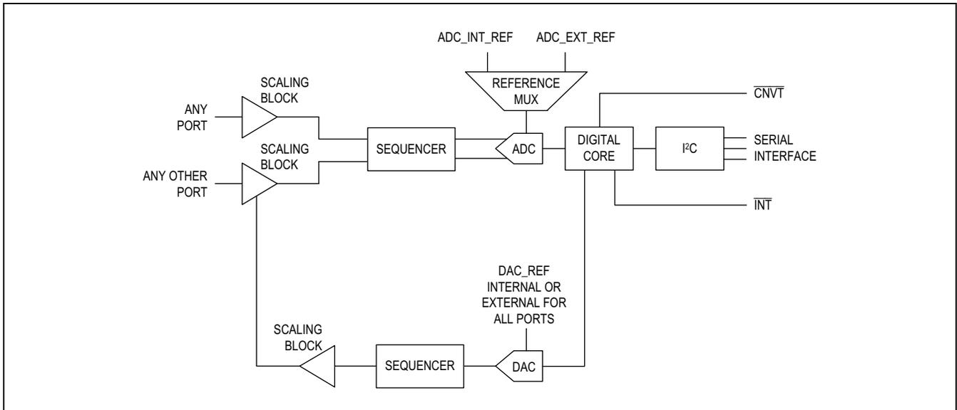
Figure 4. ADC with Pseudo-Differential Input Set by DAC
