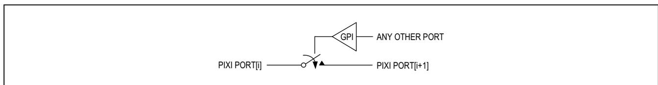
Figure 11. PIXI Ports as a Controllable Analog Switch
