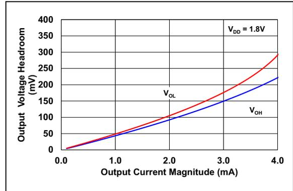
**FIGURE 2-16:** Output Voltage Headroom vs. Output Current.
