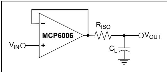
**FIGURE 4-6:** Output Resistor,  $R_{ISO}$ , Stabilizes Large Capacitive Loads.
