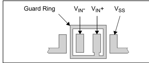
**FIGURE 4-7:** Example Guard Ring Layout for Inverting Gain.
