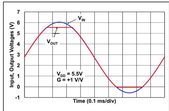
**FIGURE 2-37:** The MCP6006/6R/6U/7/9 Device Shows No Phase Reversal.
