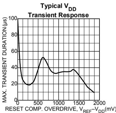
Figure 2b. Typical V<sub>DD</sub> Transient Response
