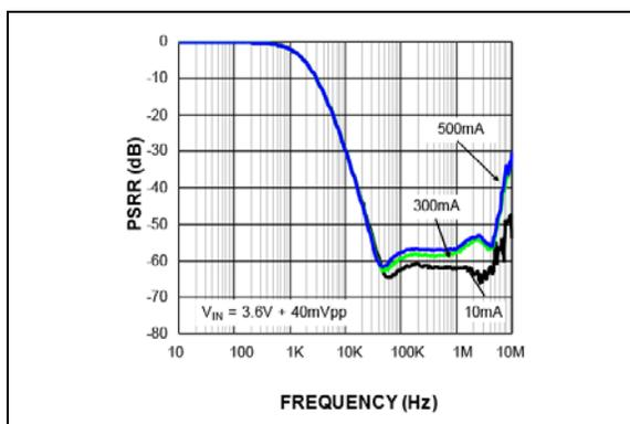
**FIGURE 2-3:** PSRR  $C_{OUT} = 4.7 \mu F$ .
