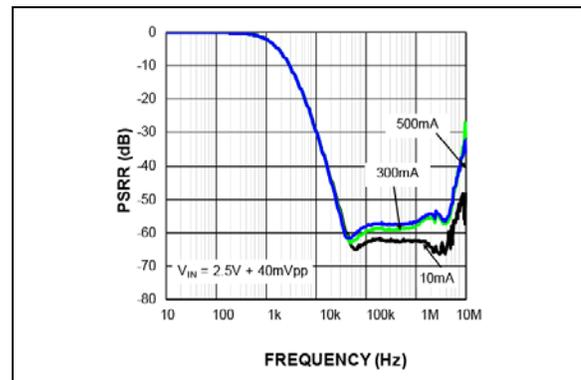
**FIGURE 2-5:** PSRR  $C_{OUT} = 10 \mu F$ .
