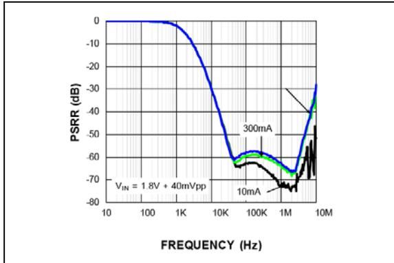
**FIGURE 2-7:** PSRR  $C_{OUT} = 22 \mu F$ .
