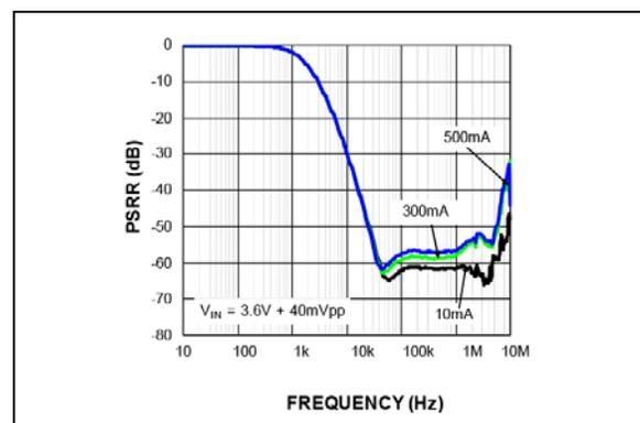
**FIGURE 2-6:** PSRR  $C_{OUT} = 10 \mu F$ .
