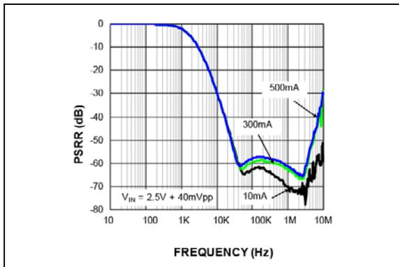
**FIGURE 2-8:** PSRR  $C_{OUT} = 22 \mu F$ .
