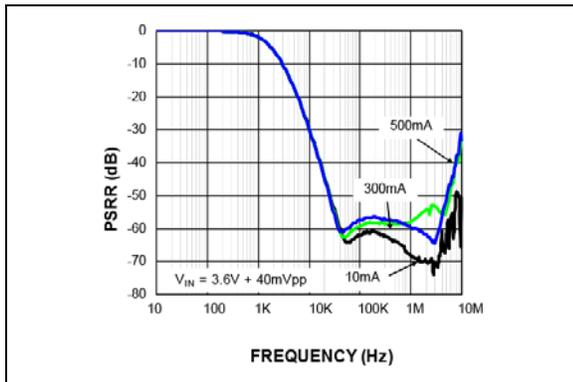
**FIGURE 2-9:** PSRR  $C_{OUT} = 22 \mu F$ .
