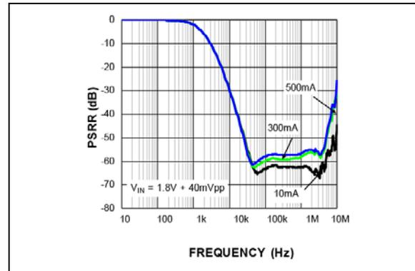
**FIGURE 2-4:** PSRR  $C_{OUT} = 10 \mu F$ .
