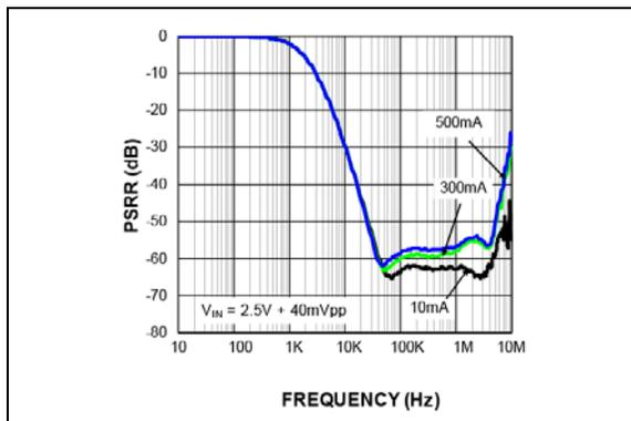
**FIGURE 2-2:** PSRR  $C_{OUT} = 4.7 \mu F$ .
