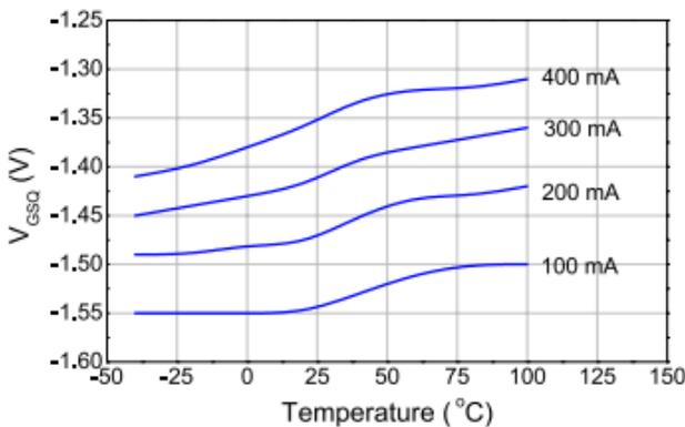
**Figure 6 - Quiescent Gate Voltage ( $V_{GSQ}$ ) Required**
