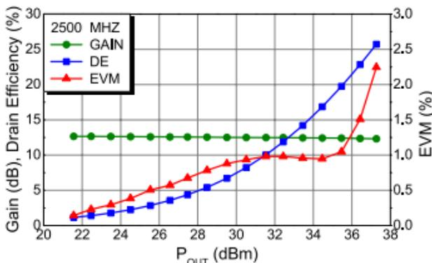
**Figure 4 - OFDM Performance Tuned for**
