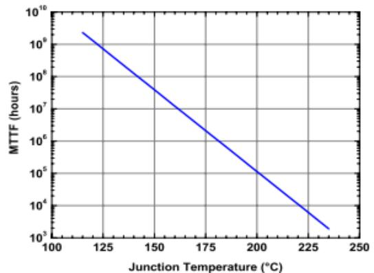
**Figure 7 - MTTF of NRF1 devices as a**
