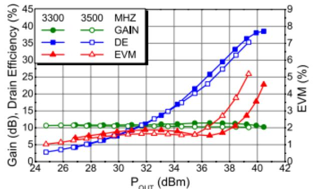
**Figure 5 - OFDM Performance Tuned for**
