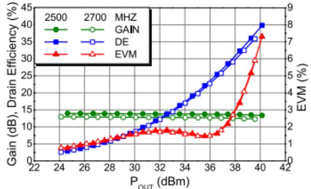
**Figure 3 - OFDM Performance Tuned for**
