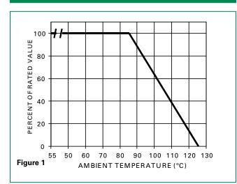
For applications exceeding 85°C ambient temperature, the peak surge current and energy ratings must be reduced as shown above.
