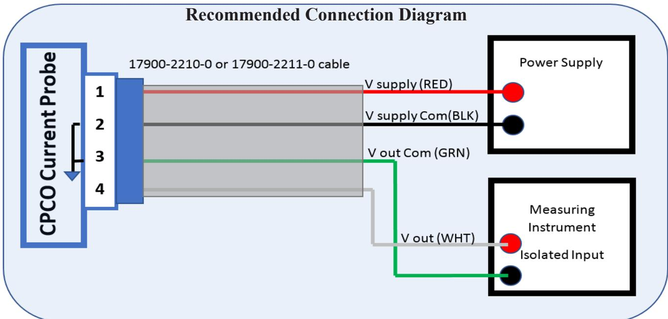
**BP10 Option** - The BP stands for Bi Polar and the output voltage from the CPCO will have a quiescent output voltage of 0.0V when there is no primary current ( $I_p=0A$ ). As the primary current ( $I_p$ ) increases in a positive direction, the output voltage will increase to the maximum level of 10.0V at  $I_p=+I_{PSAT}$ . When the primary current increases in the negative direction, the output voltage will decrease toward -10.0V at  $I_p=-I_{PSAT}$ . See below output characteristics.
