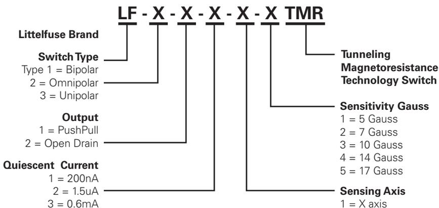
Example: LF21235TMR is an Omnipolar, PushPull, 1.5uA, X axis, 17 Gauss
