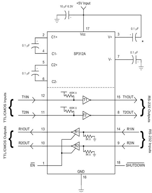
\* The Negative terminal of the V+ storage capacitor can be tied to either Vcc or GND. Connecting the capacitor to Vcc is recommended.
