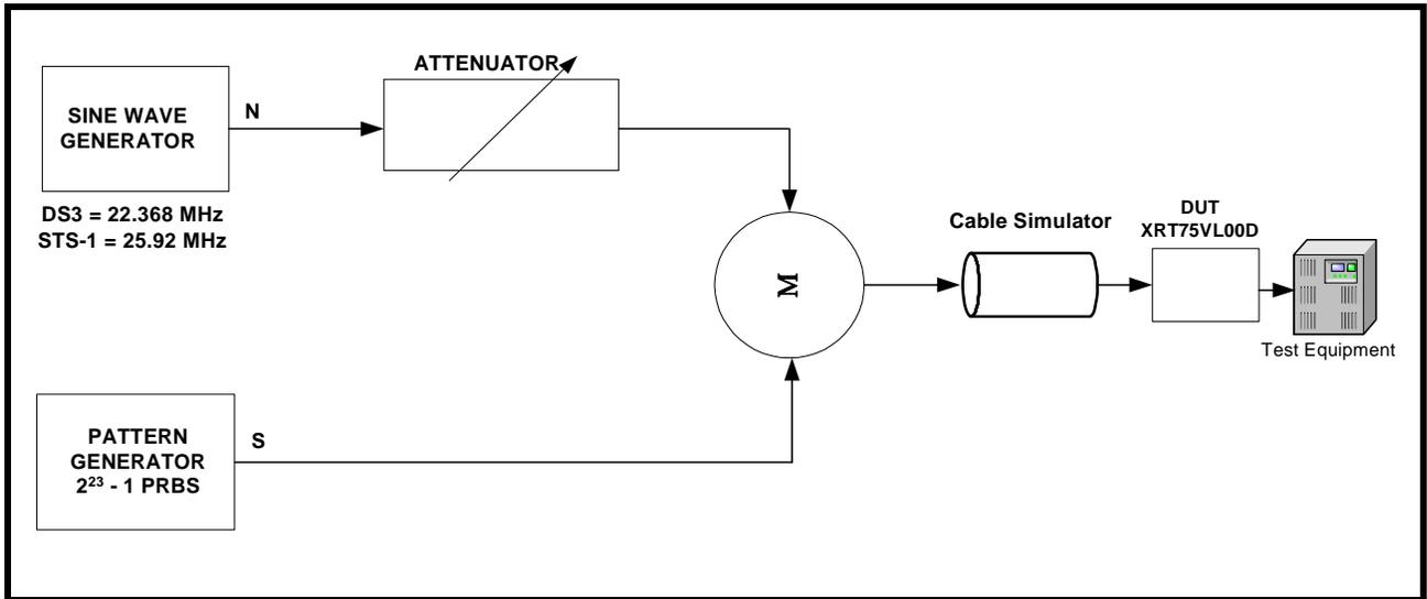
FIGURE 18. INTERFERENCE MARGIN TEST SET UP FOR E3.
