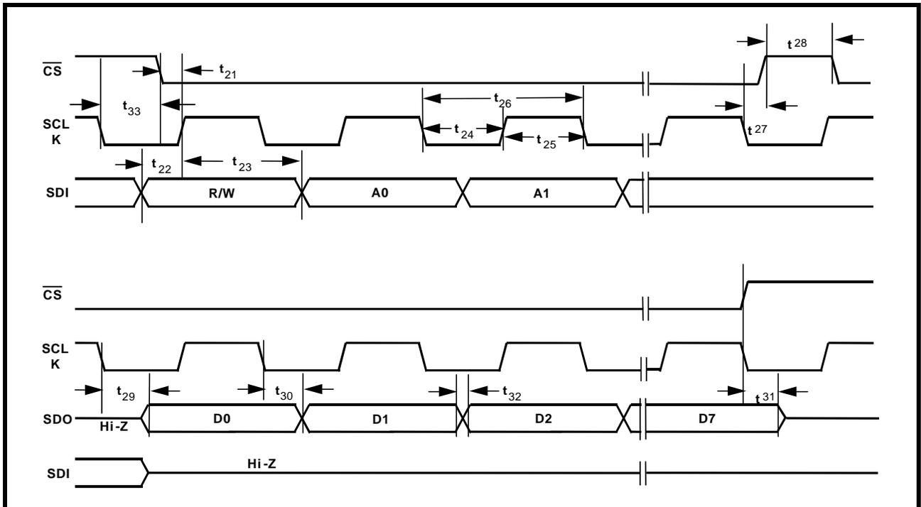
**TABLE 8: MICROPROCESSOR SERIAL INTERFACE TIMINGS (  $T_A = 25^{\circ}\text{C}$ ,  $V_{DD}=3.3\text{V}\pm 5\%$  AND LOAD = 10PF)**
