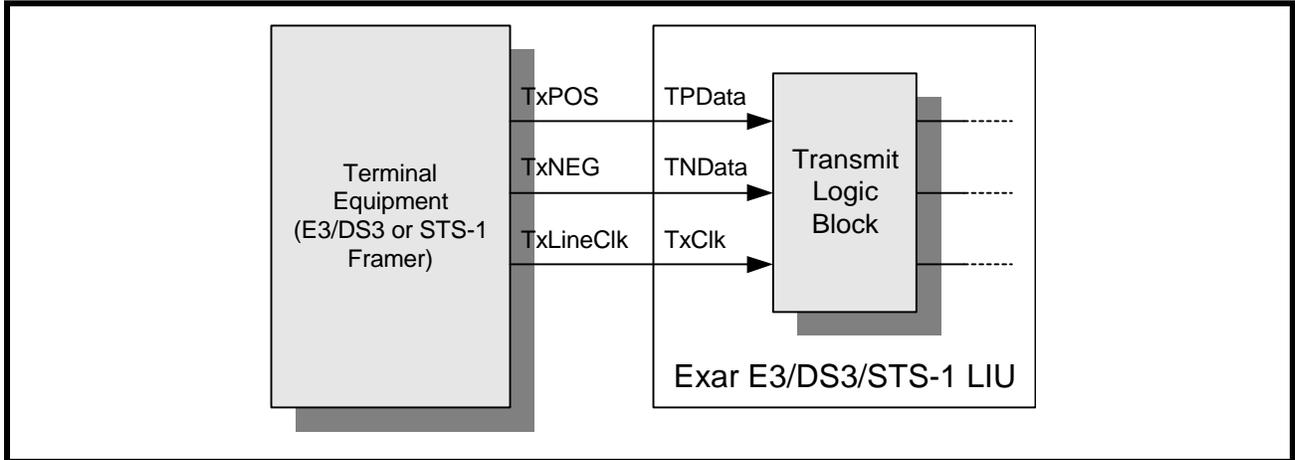
FIGURE 4. TRANSMITTER TERMINAL INPUT TIMING
