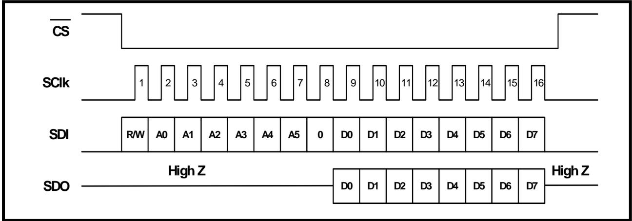
**FIGURE 11. TIMING DIAGRAM FOR THE MICROPROCESSOR SERIAL INTERFACE**
